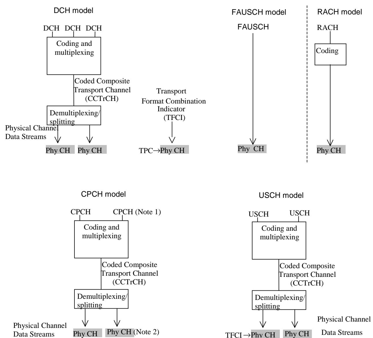
**Figure 2: Model of the UE's physical layer – uplink**
