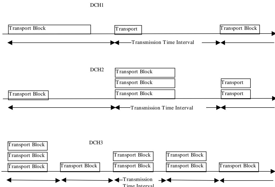
**Figure 6: Exchange of data between MAC and L1**
