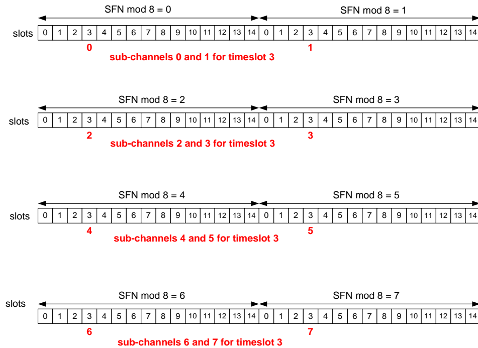
Figure 6: Eight sub-channels for timeslot 3
