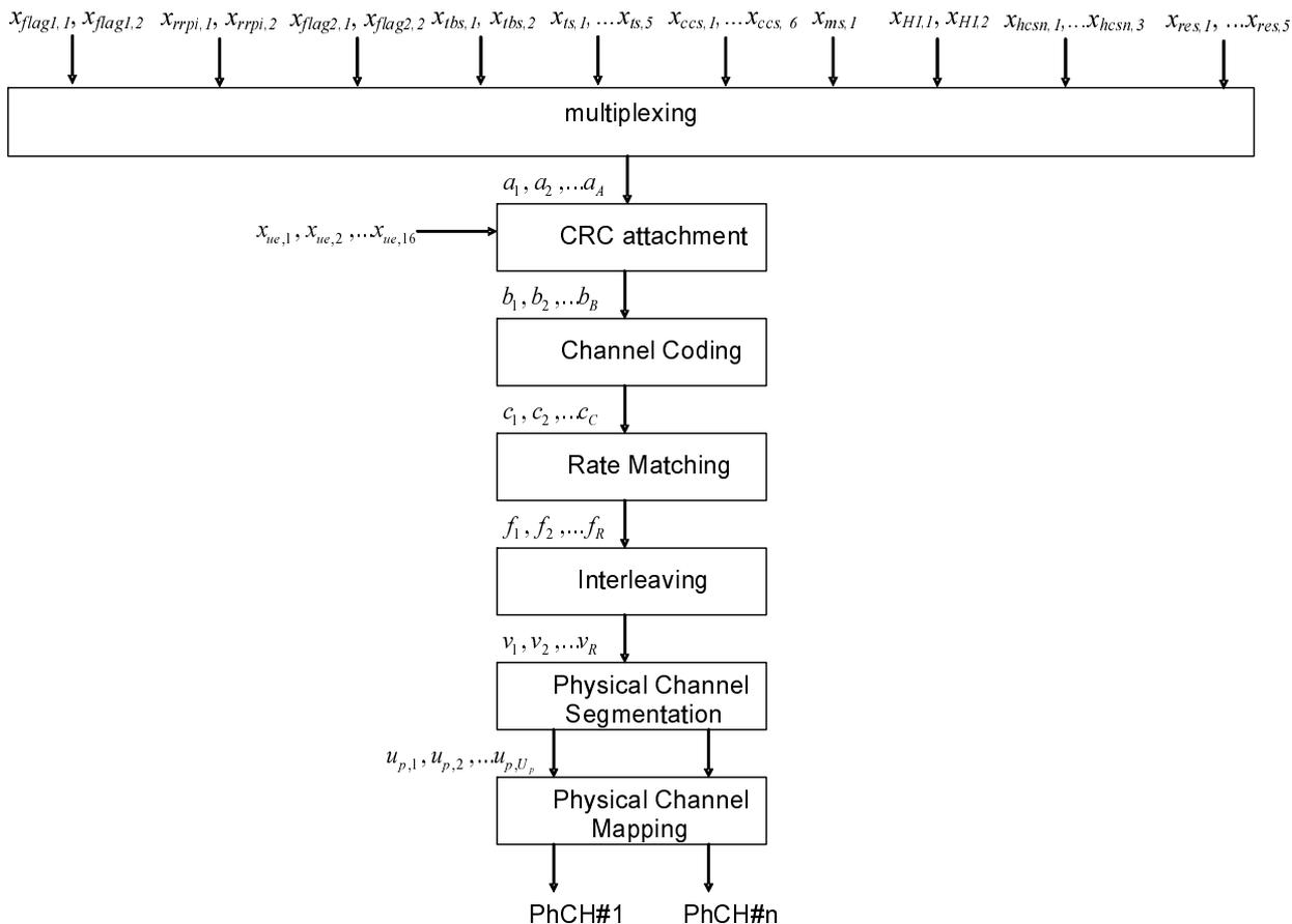
Figure 19A: Coding and Multiplexing for HS-SCCH type 2
