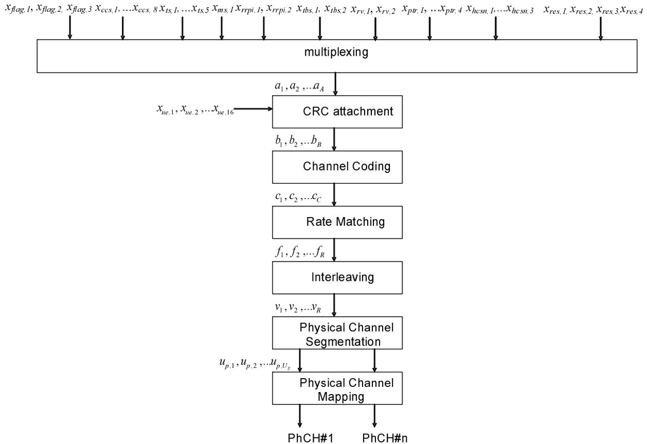
Figure 19F: Coding and Multiplexing for HS-SCCH type 7
