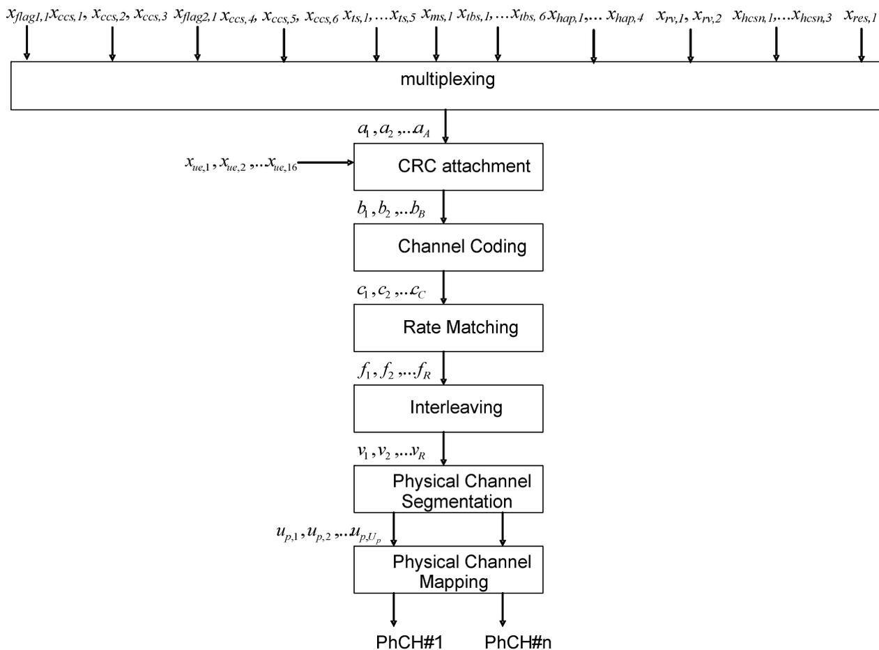
Figure 19C: Coding and Multiplexing for HS-SCCH type 4
