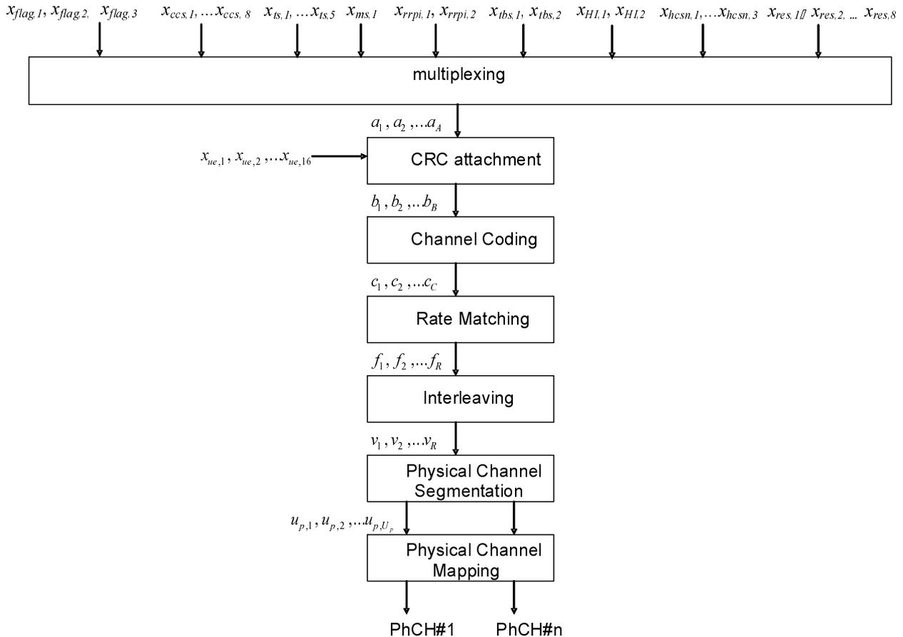
Figure 19E: Coding and Multiplexing for HS-SCCH type 6
