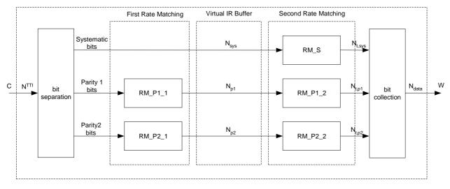
Figure 17: HS-DSCH hybrid ARQ functionality
