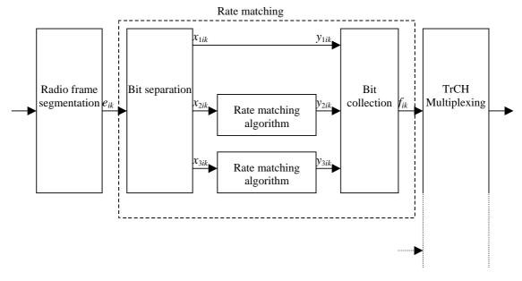
Figure 5: Puncturing of turbo encoded TrCHs
