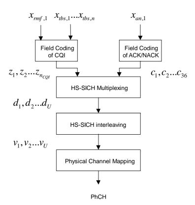
Figure 19 Coding and multiplexing for HS-SICH
