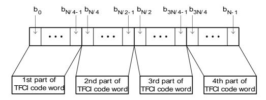
Figure 10: Mapping of TFCI code word bits to TFCI position in 1.28 Mcps TDD option, where  $N = N_{TFCI \text{ code word}}$ .
