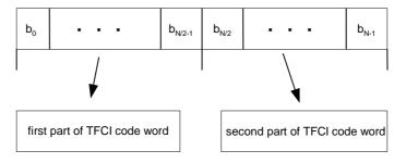
Figure 9: Mapping of TFCI code word bits to timeslot
