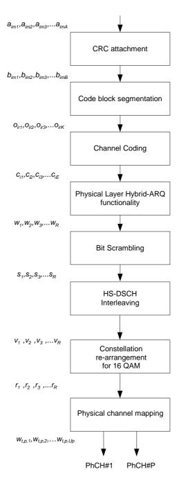
Figure 16. Coding chain for HS-DSCH
