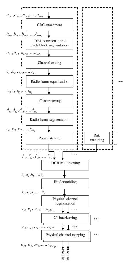
Figure 1: Transport channel multiplexing structure for uplink and downlink for 3.84Mcps TDD
