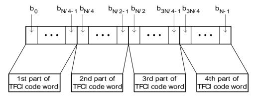
Figure 14: Mapping of TFCI code word bits to timeslot in 1.28 Mcps TDD option, where N =  $N_{TFCI \text{ code word}}$ .
