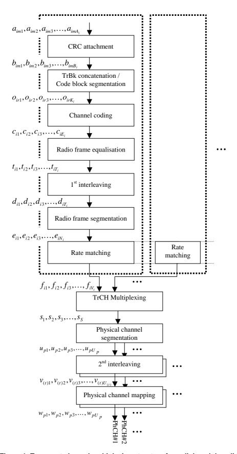
Figure 1: Transport channel multiplexing structure for uplink and downlink
