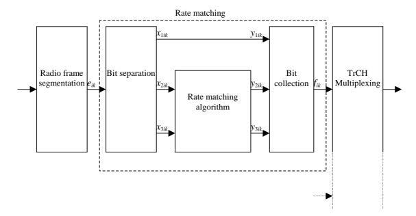
Figure 4: Puncturing of turbo encoded TrCHs
