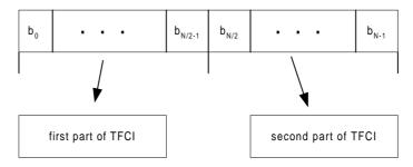
Figure 8: Mapping of TFCI word bits to timeslot
