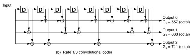
Figure 2: Rate 1/2 and rate 1/3 convolutional coders
