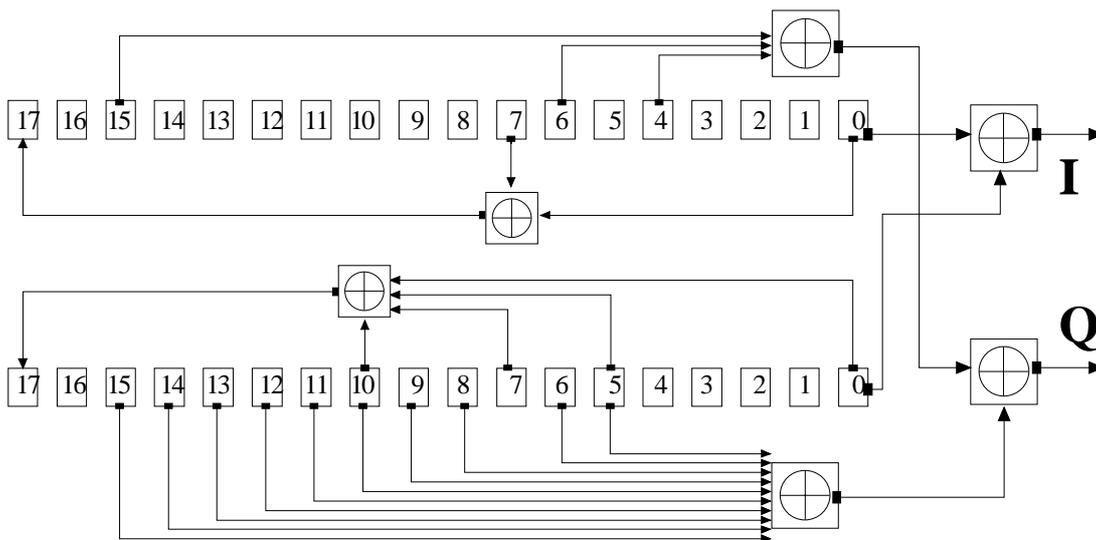
Figure 10: Configuration of downlink scrambling code generator
