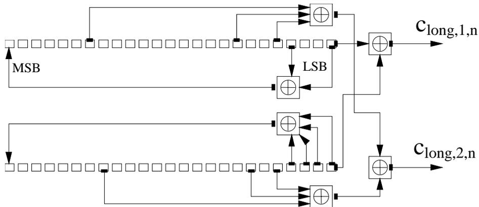
Figure 5: Configuration of uplink scrambling sequence generator
