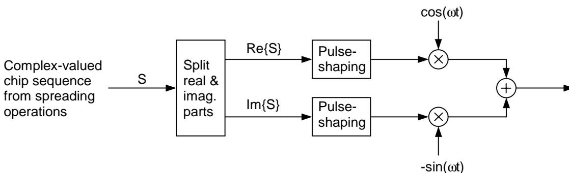
Figure 7: Uplink modulation
