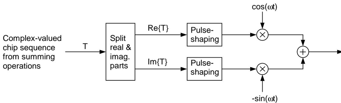
Figure 11: Downlink modulation
