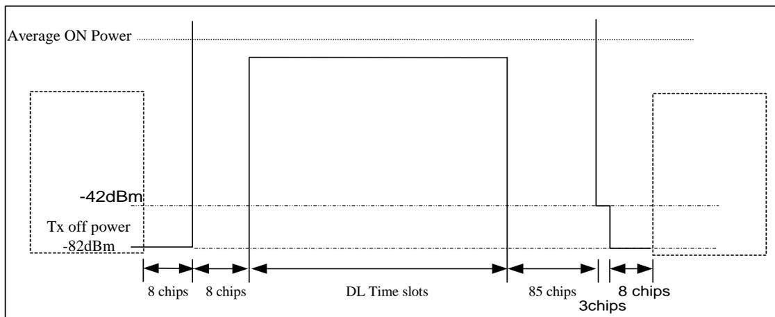
**Figure 6.1A: Transmit ON/OFF template for 1,28 Mcps TDD option**
