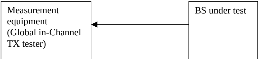
Figure B.2: Measurement system set up for RF frequency, several code power tests and transmit modulation (EVM, RCDE and PCDE)
