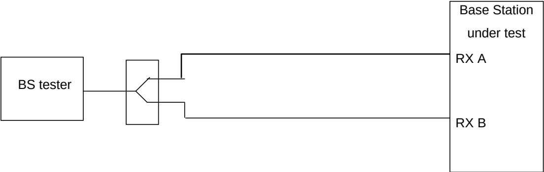
Figure B.15: Functional Set-up for Verification of the internal BLER calculation for BS with Rx diversity
