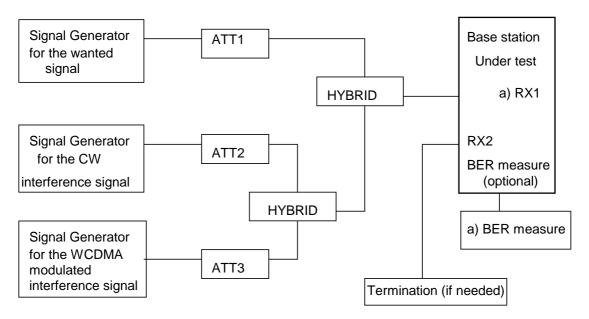
Figure B.11: Measuring system Set-up for intermodulation characteristics
