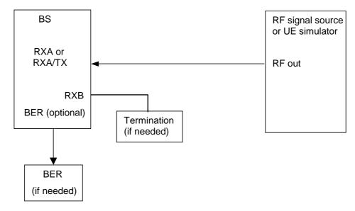
Figure B.7: Measuring system Set-up for Base Station Reference sensitivity level Testes
