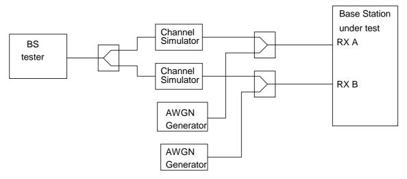
Figure B.14: Functional Set-up for Demodulation of DCH, RACH and HS-DPCCH in multipath fading conditions for BS with Rx diversity
