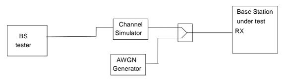
Figure B.20: Functional Set-up for Demodulation of DCH in moving propagation conditions or birthdeath propagation conditions, or Demodulation of DCH, RACH in high speed train conditions for BS without Rx diversity
