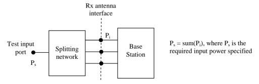
Figure 4.1: Receiver test set-up
