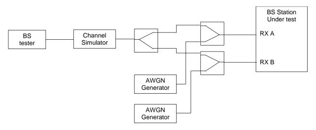
Figure B.19: Functional Set-up for Demodulation of DCH in moving propagation conditions or birthdeath propagation conditions, or Demodulation of DCH, RACH in high speed train conditions for BS with Rx diversity
