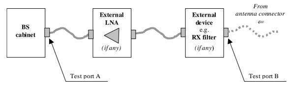
Figure 7.1: Receiver test ports
