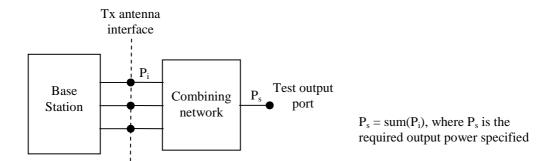
Figure 4.2: Transmitter test set-up
