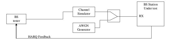
NOTE: The HARQ feedback could be done as an RF feedback or as a digital feedback. The HARQ feedback should be error free.
