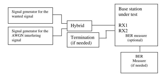
Figure B.8: Measuring system Set-up for Dynamic range
