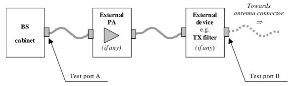
Figure 6.1: Transmitter test ports
