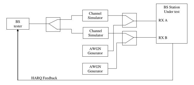
NOTE: The HARQ feedback could be done as an RF feedback or as a digital feedback. The HARQ feedback should be error free.
