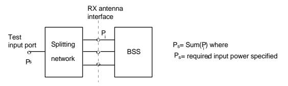
Figure 4.1: Receiver test set-up
