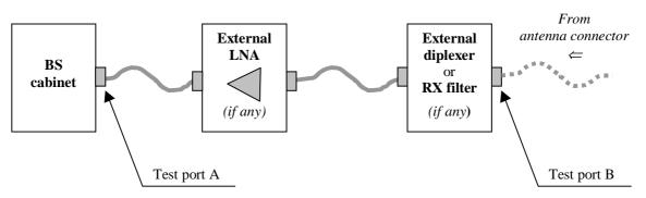
Figure 7.1: Receiver test ports
