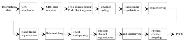
Figure 8.1: BLER insertion to the output data
