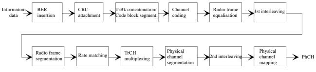
Figure 7.1: BER insertion into the information data
