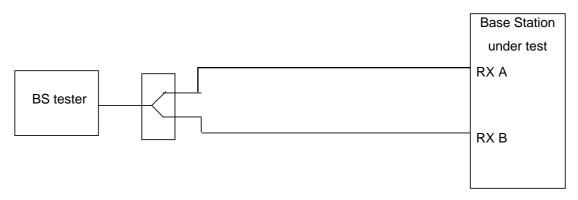
Figure B.15: Functional Set-up for Verification of the internal BLER calculation
