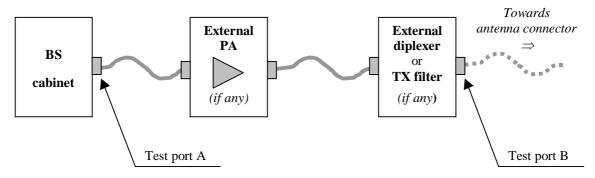
Figure 6.1: Transmitter test ports
