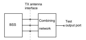
Figure 4.2: Transmitter test set-up
