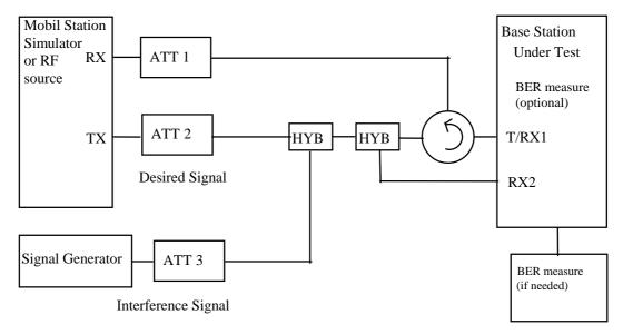
Figure B.10: Measuring system Set-up for Blocking characteristics
