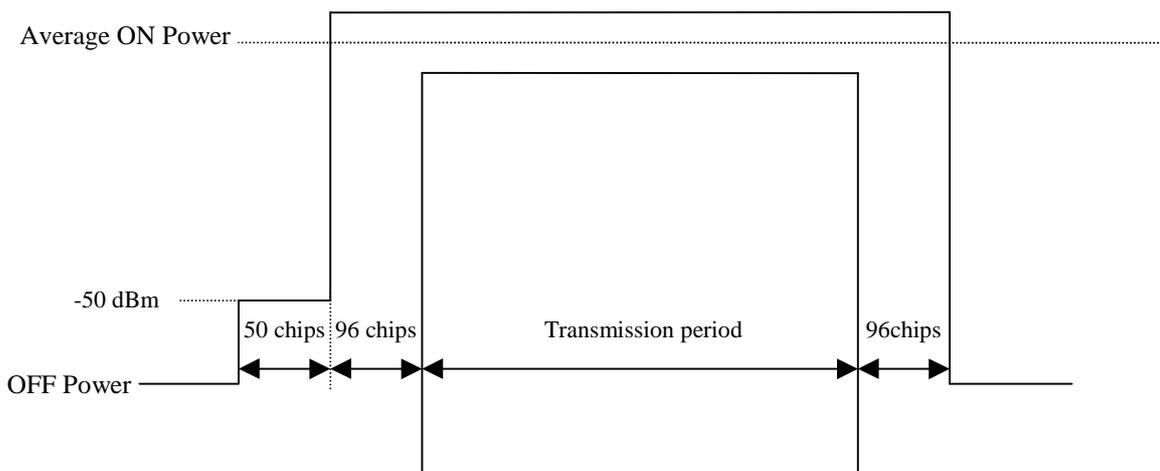
Figure 6.2: Transmit ON/OFF template for 3.84 Mcps TDD Option
