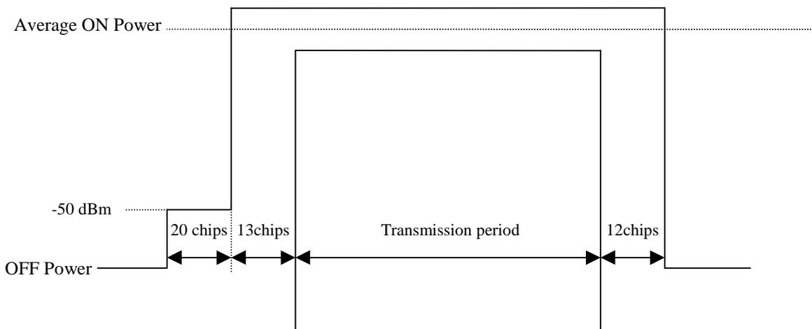
Figure 6.2A: Transmit ON/OFF template for 1.28 Mcps TDD Option
