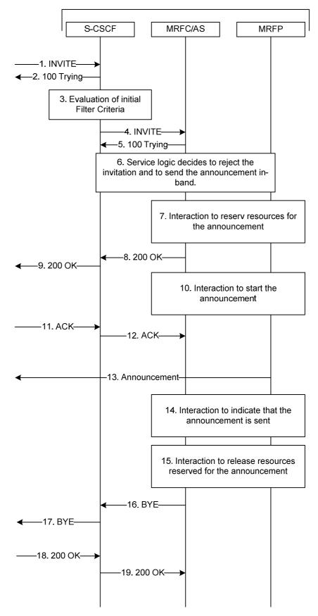
Figure A.9: In-band information generated by network when an invitation to a communication is rejected
