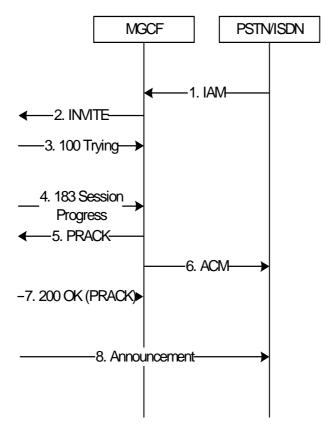
NOTE: The flow assumes the use of the option-tag "100rel" defined in RFC 3262 [5] other scenarios can also apply. T-MGF is left out of the figure for simplicity.
