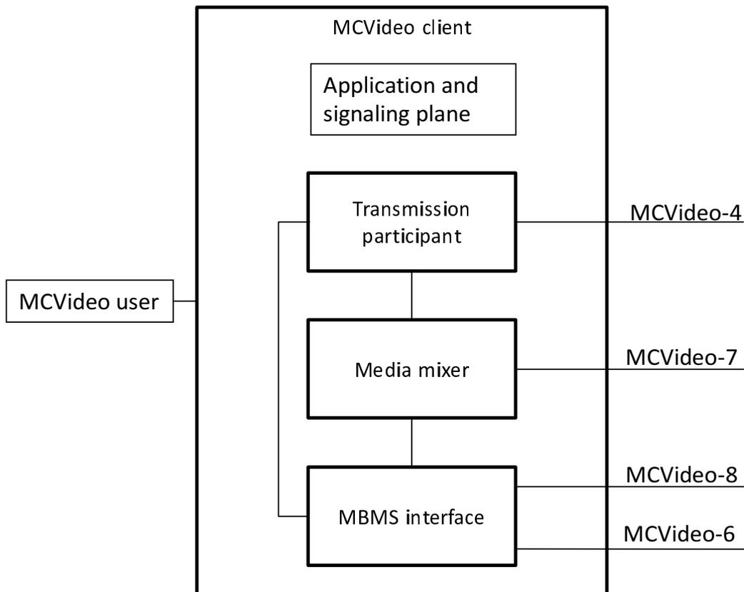
NOTE: The real internal structure of the MCVideo client is implementation specific but a possible internal structure is shown to illustrate the logic and the procedures.
