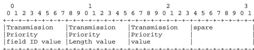
The <Transmission Priority field ID> value is a binary value and is set according to table 9.2.3.1-1.
