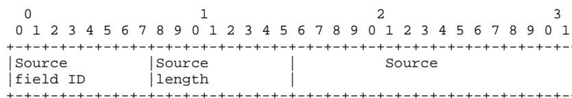
The <Source field ID> value is a binary value and is set according to table 9.2.3.1-1.
