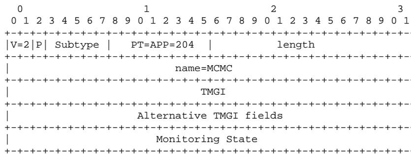
With the exception of the three first 32-bit words and the internal order of the TMGI field and the Alternative TMGI fields, the order of the fields is irrelevant.
