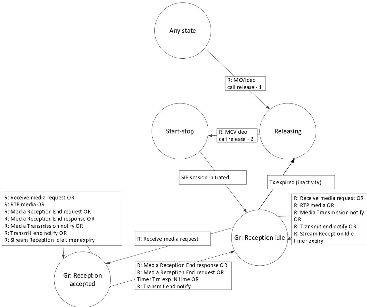
**Figure 6.3.6.1-1: Transmission control server state transition diagram for 'general reception control operation'**
