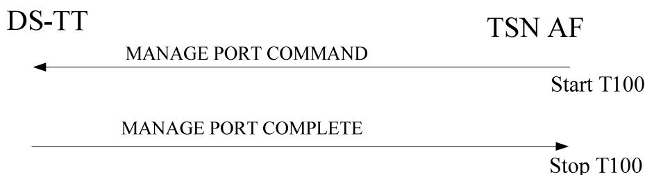
Figure 5.2.1.2.1: Network-requested port management procedure
