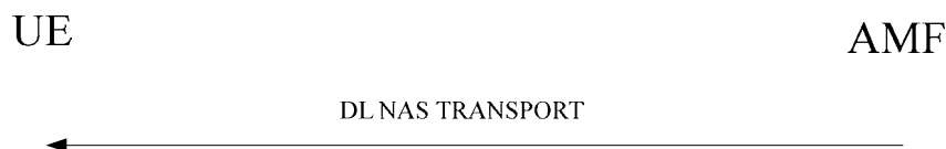
Figure 5.4.5.3.2.1: Network-initiated NAS transport procedure
