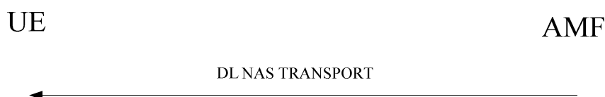
Figure 5.4.5.3.2.1: Network-initiated NAS transport procedure
