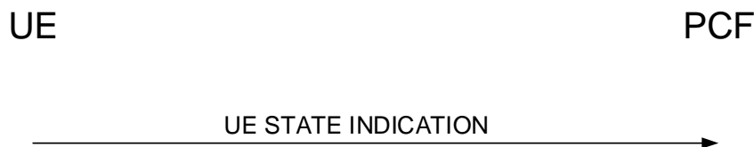
Figure D.2.2.2.1: UE-initiated UE state indication procedure
