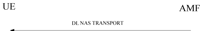
Figure 5.4.5.3.2.1: Network-initiated NAS transport procedure
