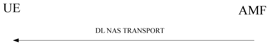
Figure 5.4.5.3.2.1: Network-initiated NAS transport procedure
