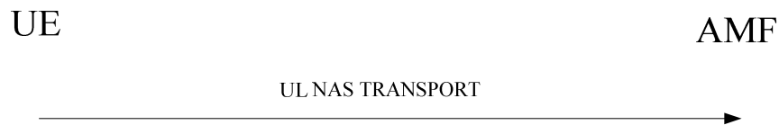
Figure 5.4.5.2.2.1: UE-initiated NAS transport procedure
