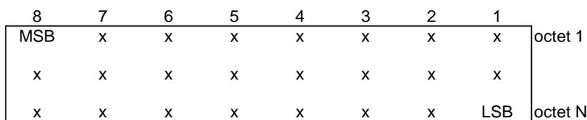
**Figure 15.2.1-1: Example of bit ordering of a field**
