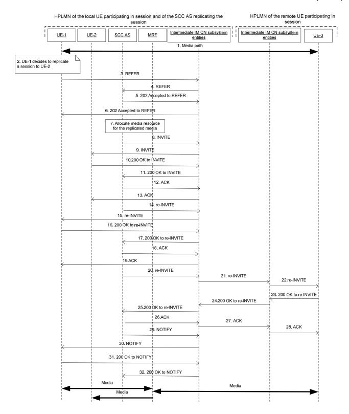
Figure A.12.3-1: Signalling flow for replicating media in network from controller to another UE- push mode
