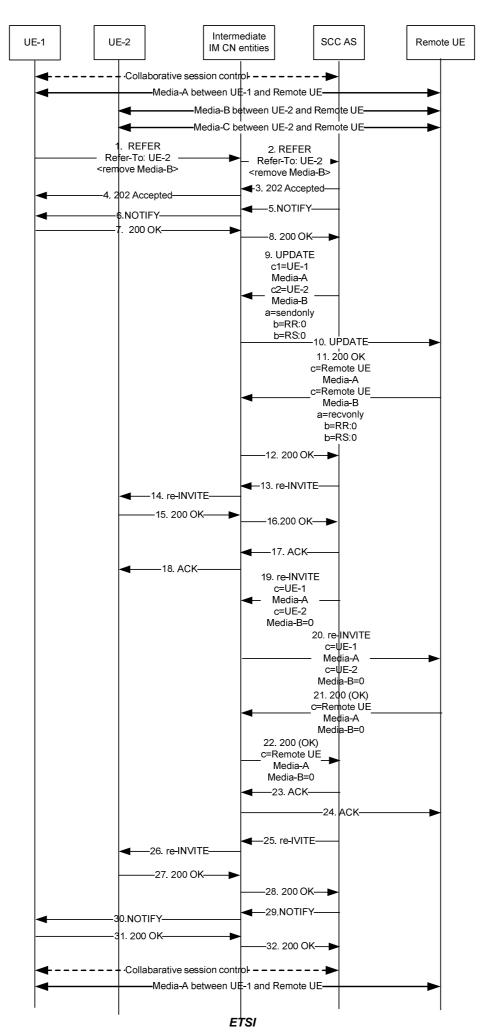
NOTE 1: For clarity, the SIP 100 (Trying) responses are not shown in the signalling flow. **Figure A.7.2.2.1:Controller UE remove media at the controllee UE**
