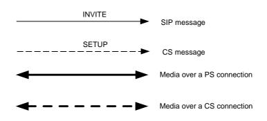
Figure A.2-1: Signalling flow notation
