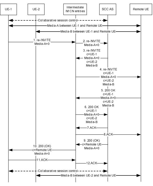
Figure A.7.2.1: Controller UE releases media flow on controller UE
