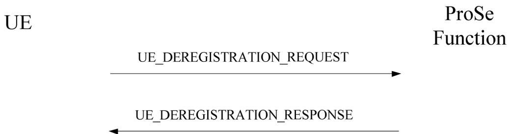
**Figure 7.2.6.2.1.1: UE-initiated UE deregistration procedure**
