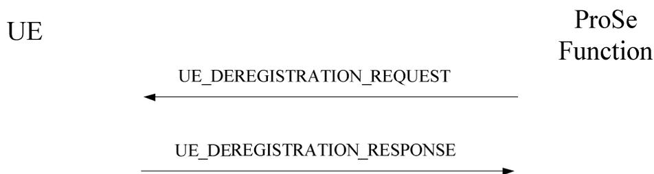
**Figure 7.2.6.3.1.1: Network-initiated UE deregistration procedure**
