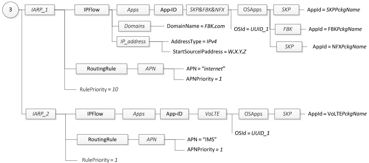
**Figure C.3.3.3: IARP InterAPNRouting flow distribution rules for roaming**
