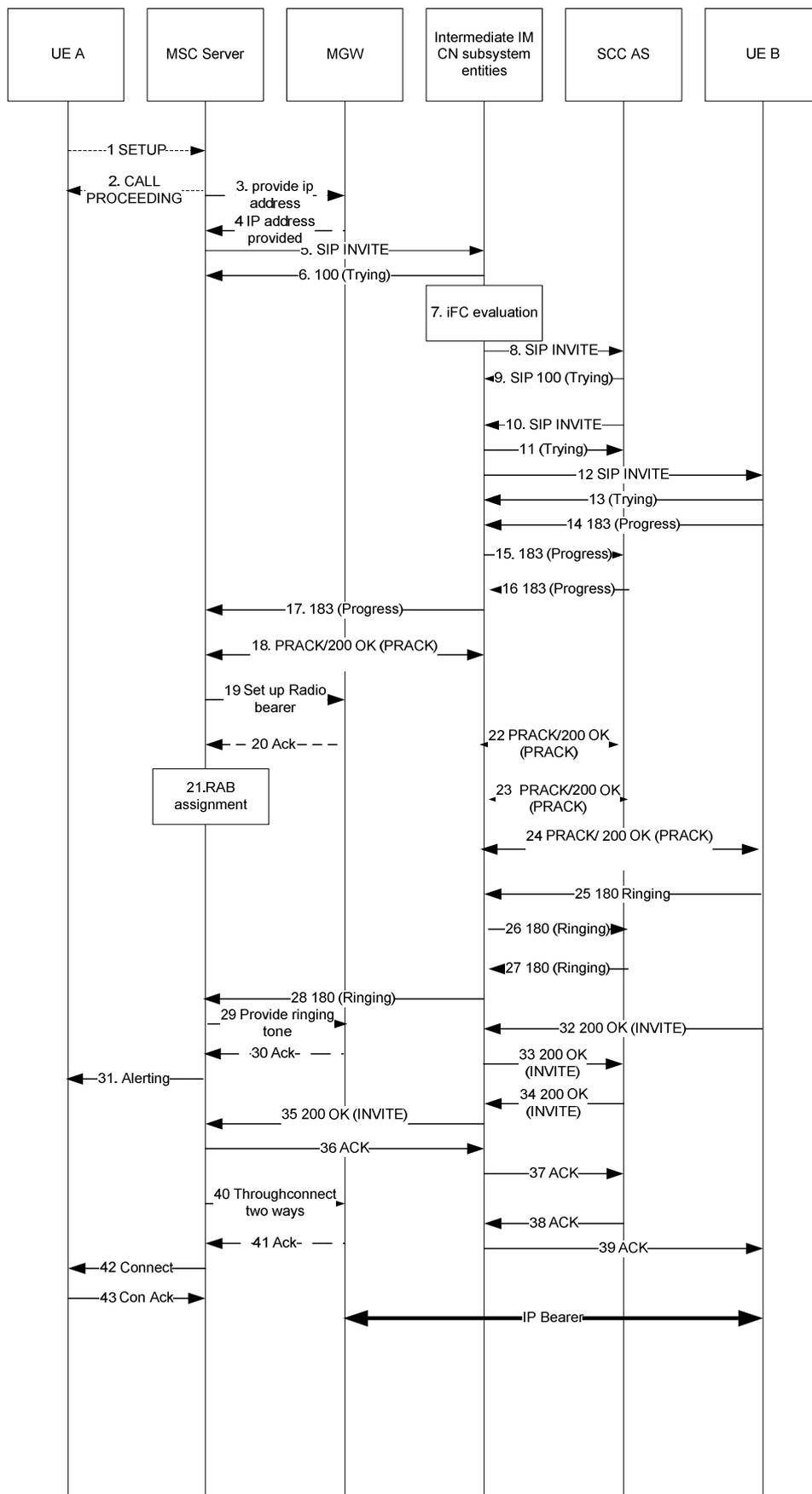
Figure A.4.3-1: CS UE Origination with CS media using Gm reference point when using an MSC Server enhanced for ICS
