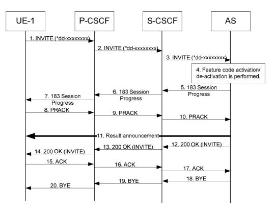
Figure A-2: User provisioning using feature code
