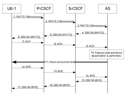
Figure A-1: User provisioning using feature code
