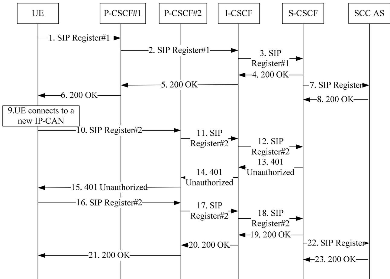
Figure A.3.2-1 Signalling flows for multiple registrations
