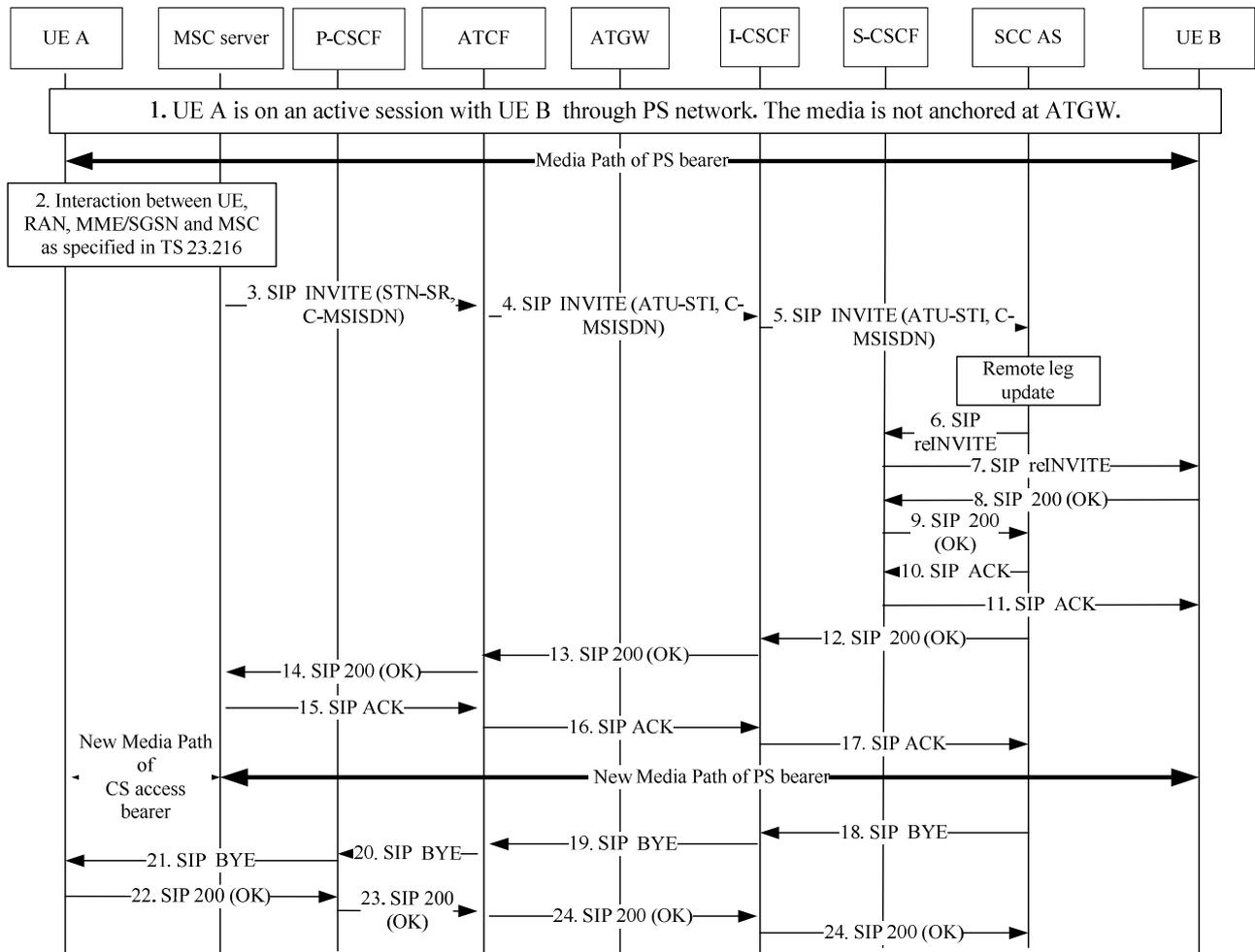
**Figure A.18.2-1 Signalling flows for PS to CS access transfer: PS to CS SRVCC enhancements using ATCF and without media anchored**
