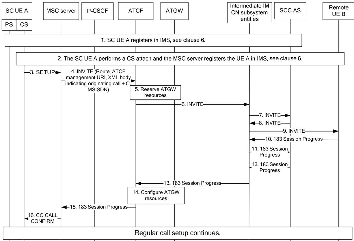
NOTE: For clarity, the SIP 100 (Trying) responses are not shown in the signalling flow.
