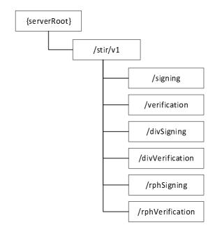
Figure V.2.2-1: Resource structure for the resource exposed over the Ms reference point
