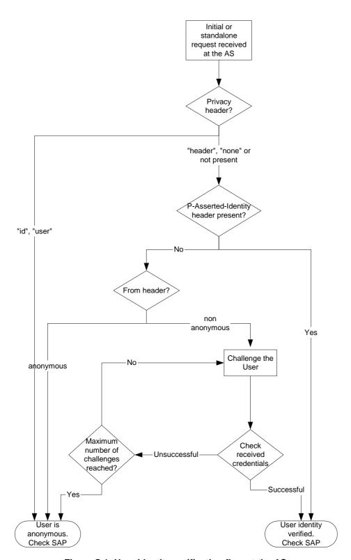
Figure 5-1: User identity verification flow at the AS
