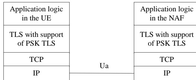
Figure 5.3.1-2: Protocol stack of Ua interface with PSK TLS
