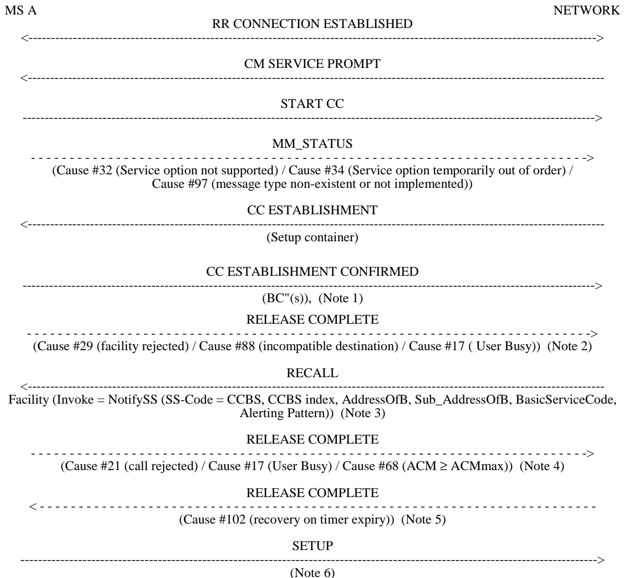
Figure 4.3.1: CCBS Call Set-up for supporting MSs - subscriber A idle when RECALL arrives
