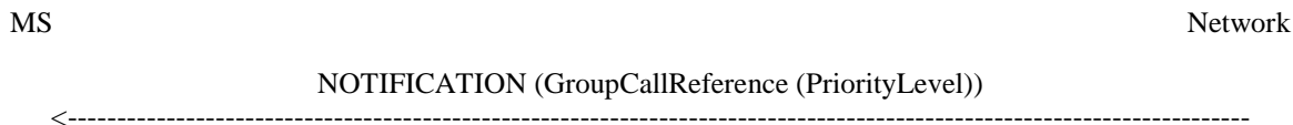
Figure 5: Signalling information between the network and the called mobile stations required for the prioritisation in case of a VGCS or VBS call
