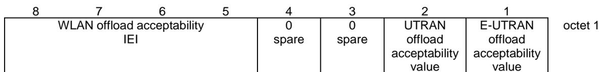
**Figure 10.5.6.20-1/3GPP TS 24.008: *WLAN offload acceptability* information element**
