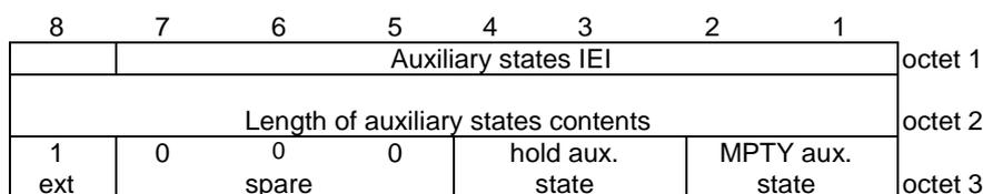
**Figure 10.5.87/3GPP TS 24.008 Auxiliary states information element**
