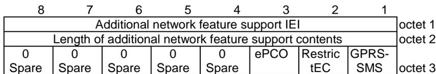
**Figure 10.5.5.23A: Additional network feature support information element**
