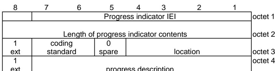
**Figure 10.5.107/3GPP TS 24.008 Progress indicator information element**
