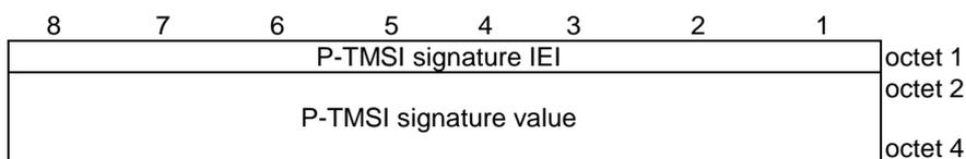
**Figure 10.5.124/3GPP TS 24.008: P-TMSI signature information element****Table 10.5.141/3GPP TS 24.008: P-TMSI signature information element**
