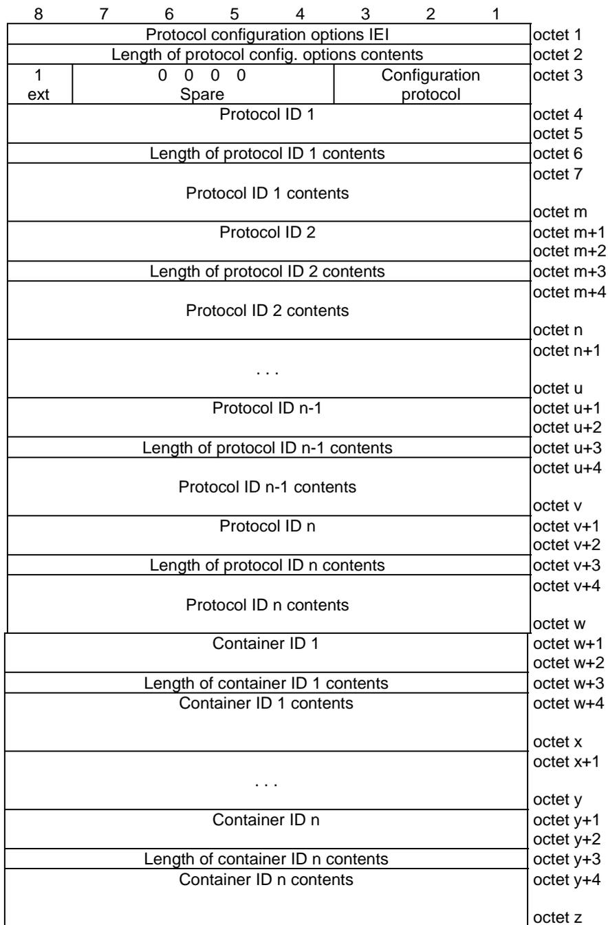
Figure 10.5.136/3GPP TS 24.008: Protocol configuration options information element
