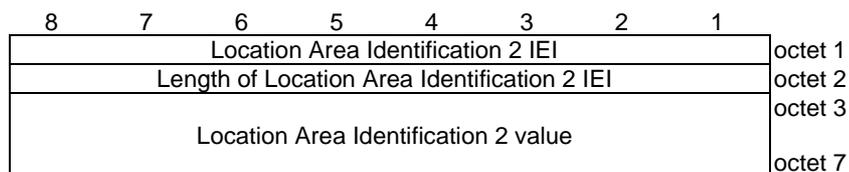
**Figure 10.5.5.30/3GPP TS 24.008: Location Area Identification 2 information element**
