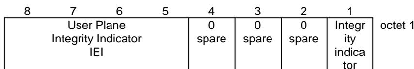
**Figure 10.5.5-1/3GPP TS 24.008 User Plane integrity indicator information element**
