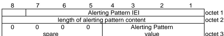
Figure 10.5.115/3GPP TS 24.008 Alerting Pattern information element
