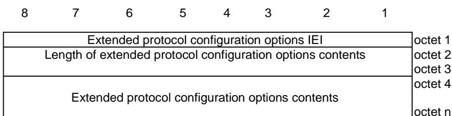
**Figure 10.5.6.3A.1: Extended protocol configuration options information element**
