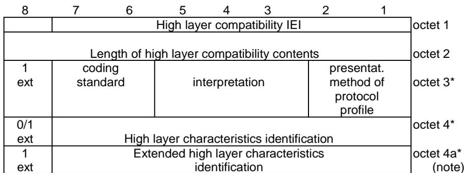
**Figure 10.5.102/3GPP TS 24.008 High layer compatibility information element**
