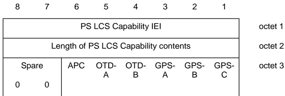
**Figure 10.5.135b/3GPP TS 24.008: PS LCS Capability information element**
