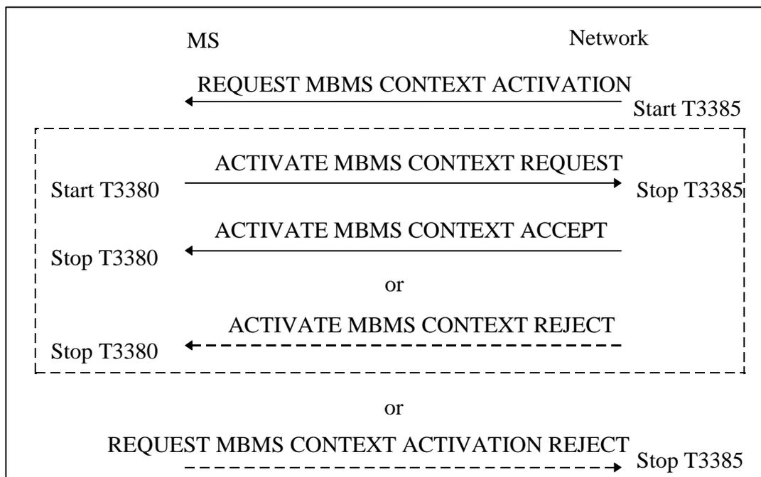
**Figure 6.10/3GPP TS 24.008: MBMS context activation procedure**
