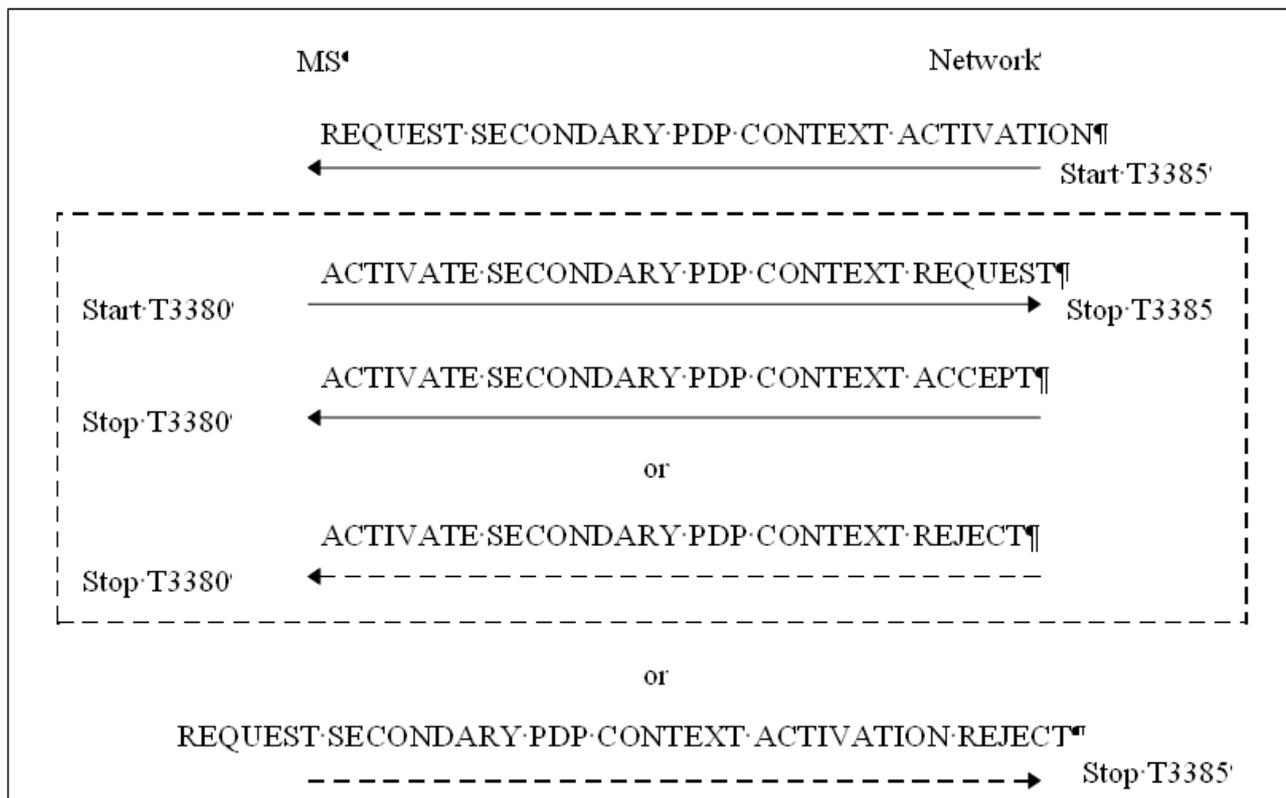
Figure 6.5a/3GPP TS 24.008: Network requested secondary PDP context activation procedure
