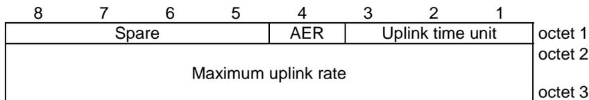
**Figure 10.5.136A/3GPP TS 24.008: APN rate control parameters**
