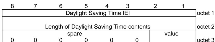
**Figure 10.5.84b/3GPP TS 24.008 *Daylight Saving Time* information element**
