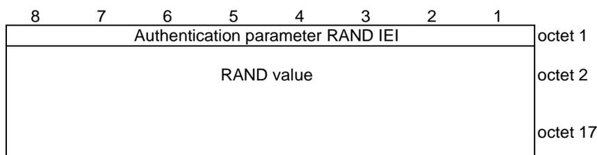
**Figure 10.5.75/3GPP TS 24.008 Authentication Parameter RAND information element**
