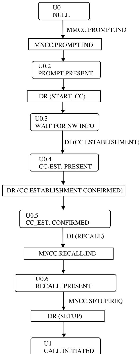
Figure 5.1a.1/3GPP TS 24.008: Overview call control protocol/MS side, extension
