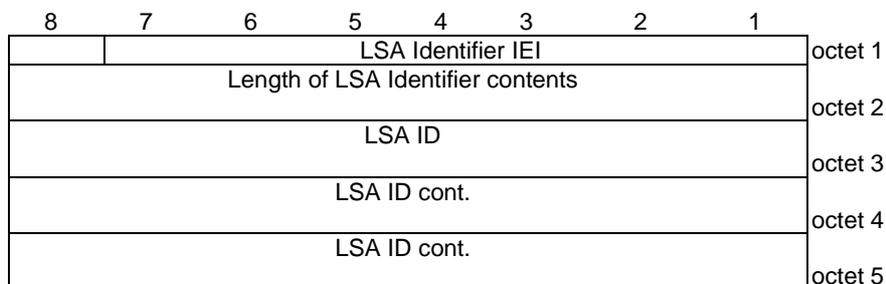
**Figure 10.68c/3GPP TS 24.008 *LSA Identifier* information element**
