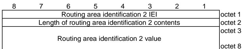
**Figure 10.5.130a/3GPP TS 24.008: Routing area identification 2 information element**
