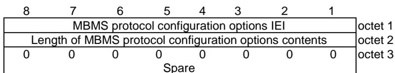
**Figure 10.5.156/3GPP TS 24.008: MBMS protocol configuration options information element**
