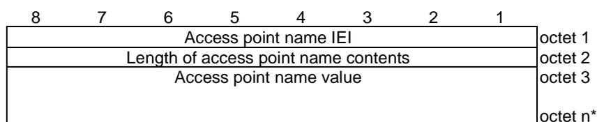
**Figure 10.5.152/3GPP TS 24.008: Access point name information element**
