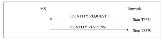
Figure 4.7.8/1 3GPP TS 24.008: Identification procedure
