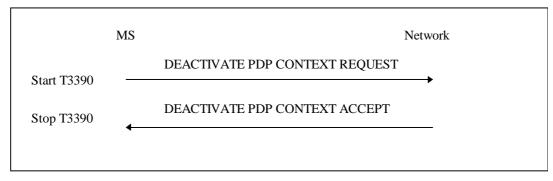
Figure 6.8/3GPP TS 24.008: MS initiated PDP context deactivation procedure
