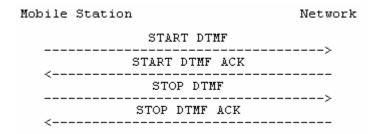
Figure 5.8/3GPP TS 24.008 Single DTMF transmission
