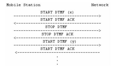
Figure 5.9/3GPP TS 24.008 Multiple DTMF transmission
