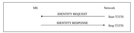
Figure 4.7.8/1 3GPP TS 24.008: Identification procedure
