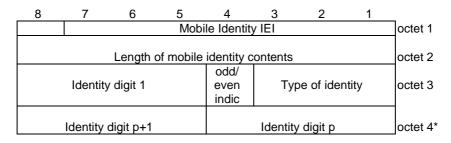
Figure 10.5.4/3GPP TS 24.008 Mobile Identity information element
