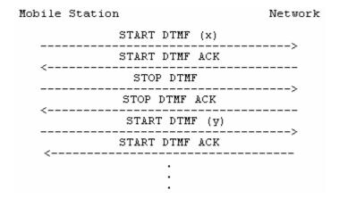
Figure 5.9/3GPP TS 24.008 Multiple DTMF transmission
