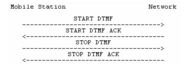
Figure 5.8/3GPP TS 24.008 Single DTMF transmission
