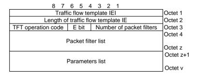
Figure 10.5.144/3GPP TS 24.008: Traffic flow template information element
