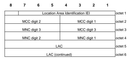
Figure 10.5.3/3GPP TS 24.008 Location Area Identification information element
