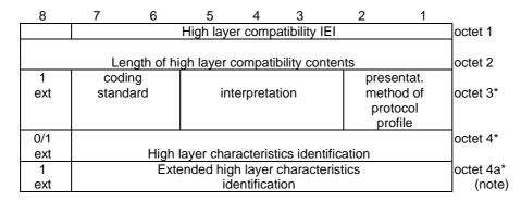
Figure 10.5.102/3GPP TS 24.008 High layer compatibility information element
