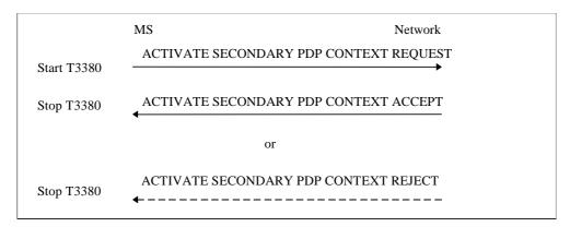
Figure 6.5/3GPP TS 24.008: MS initiated secondary PDP context activation procedure
