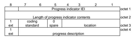
Figure 10.5.107/3GPP TS 24.008 Progress indicator information element
