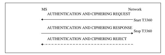
Figure 4.7.7/1 3GPP TS 24.008: Authentication and ciphering procedure
