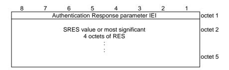
Figure 10.5.76/3GPP TS 24.008 Authentication Response Parameter information element
