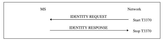
Figure 4.7.8/1 3GPP TS 24.008: Identification procedure
