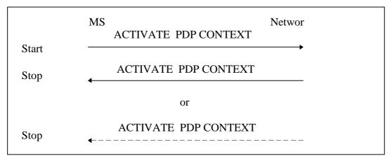
Figure 6.3/3GPP TS 24.008: MS initiated PDP context activation procedure
