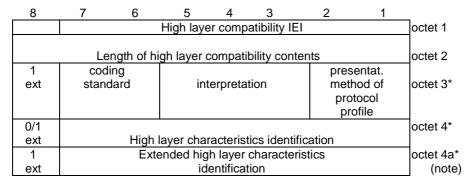
Figure 10.5.102/3GPP TS 24.008 High layer compatibility information element
