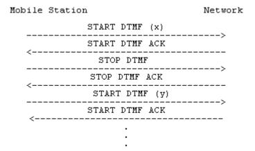
Figure 5.9/3GPP TS 24.008 Multiple DTMF transmission
