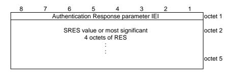
Figure 10.5.76/3GPP TS 24.008 Authentication Response Parameter information element
