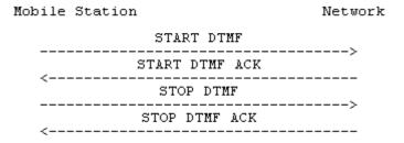
Figure 5.8/3GPP TS 24.008 Single DTMF transmission
