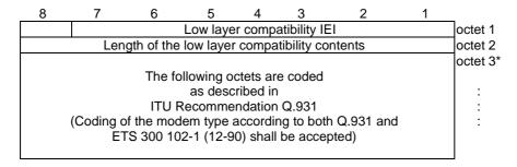
Figure 10.5.104/3GPP TS 24.008 Low layer compatibility information element
