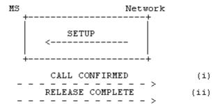
Figure 5.6/3GPP TS 24.008 Mobile terminating call initiation and possible subsequent responses.
