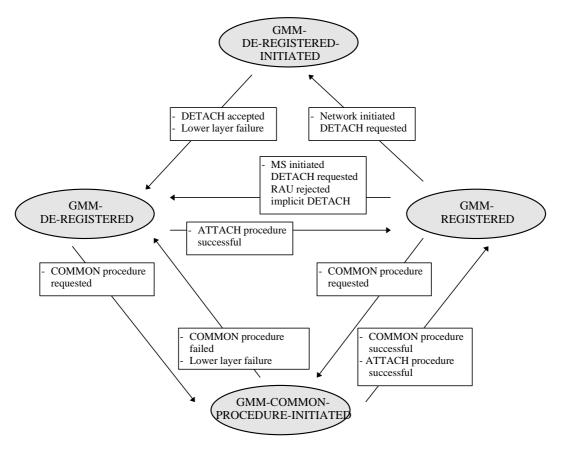
Figure 4.1c/3GPP TS 24.008: GMM main states on the network side
