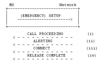
Figure 5.2/3GPP TS 24.008 Mobile originated call initiation and possible subsequent responses.
