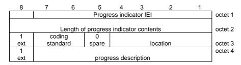
Figure 10.5.107/3GPP TS 24.008 Progress indicator information element
