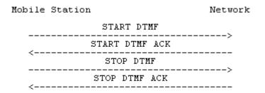
Figure 5.8/3GPP TS 24.008 Single DTMF transmission
