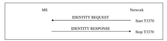
Figure 4.7.8/1 3GPP TS 24.008: Identification procedure
