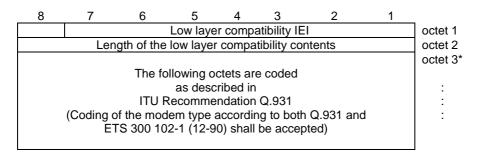
Figure 10.5.104/3GPP TS 24.008 Low layer compatibility information element
