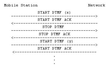
Figure 5.9/3GPP TS 24.008 Multiple DTMF transmission
