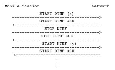
Figure 5.9/TS 24.008 Multiple DTMF transmission
