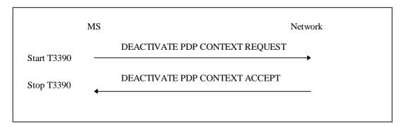
Figure 6.8/TS 24.008: MS initiated PDP context deactivation procedure
