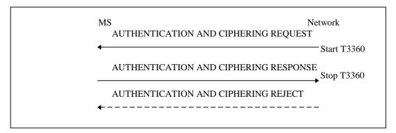
Figure 4.7.7/1 TS 24.008: Authentication and ciphering procedure
