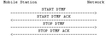
Figure 5.8/TS 24.008 Single DTMF transmission
