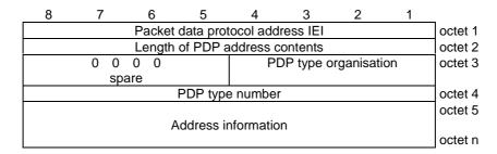
Figure 10.5.137/TS 24.008: Packet data protocol address information element
