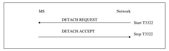
Figure 4.7.4/2 TS 24.008: Network initiated GPRS detach procedure
