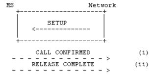
Figure 5.6/TS 24.008 Mobile terminating call initiation and possible subsequent responses.
