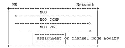
Figure 5.10b/TS 24.008 In-call modification sequence initiated by network
