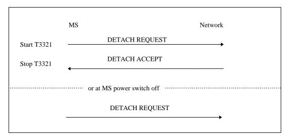
Figure 4.7.4/1 TS 24.008: MS initiated GPRS detach procedure
