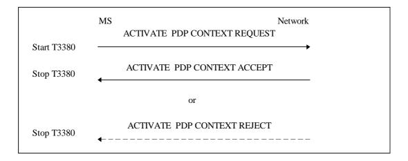
Figure 6.3/TS 24.008: MS initiated PDP context activation procedure
