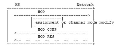
Figure 5.10a/TS 24.008 In-call modification sequence initiated by MS
