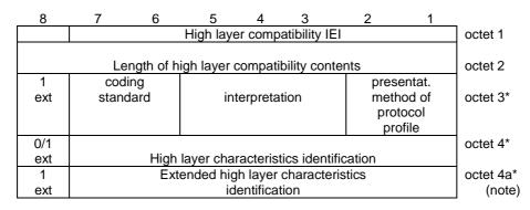
Figure 10.5.102/TS 24.008 High layer compatibility information element
