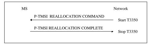
Figure 4.7.6/1 TS 24.008: P-TMSI reallocation procedure
