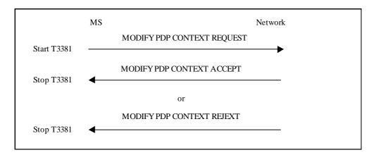
Figure 6.7/TS 24.008: MS initiated PDP context modification procedure
