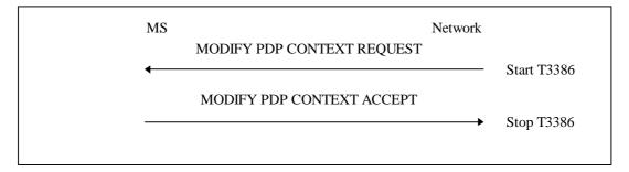
Figure 6.6/TS 24.008: Network initiated PDP context modification procedure
