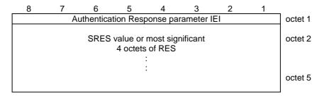
Figure 10.5.76/TS 24.008 Authentication Response Parameter information element
