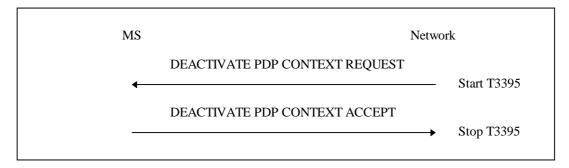
Figure 6.9/TS 24.008: Network initiated PDP context deactivation procedure
