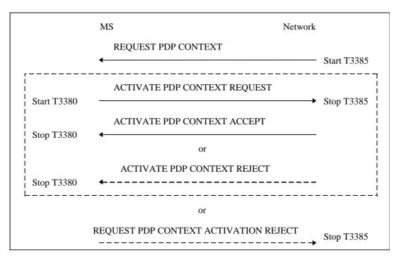
Figure 6.4/TS 24.008: Network initiated PDP context activation procedure
