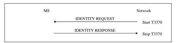
Figure 4.7.8/1 TS 24.008: Identification procedure
