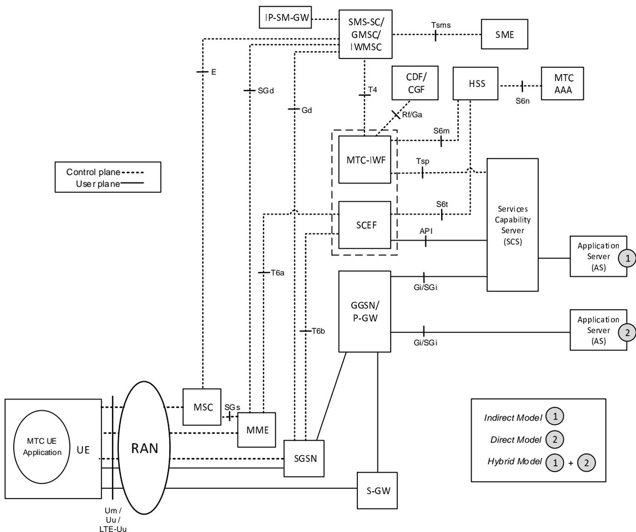
Figure 4.2-1a: 3GPP Architecture for Machine-Type Communication (non-roaming)
