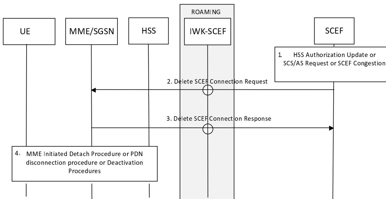
**Figure 5.13.5.3-1: SCEF Initiated T6a/T6b Connection Release procedure**
