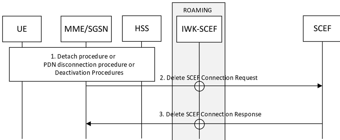
**Figure 5.13.5.2-1: MME/SGSN Initiated T6a/T6b Connection Release procedure**
