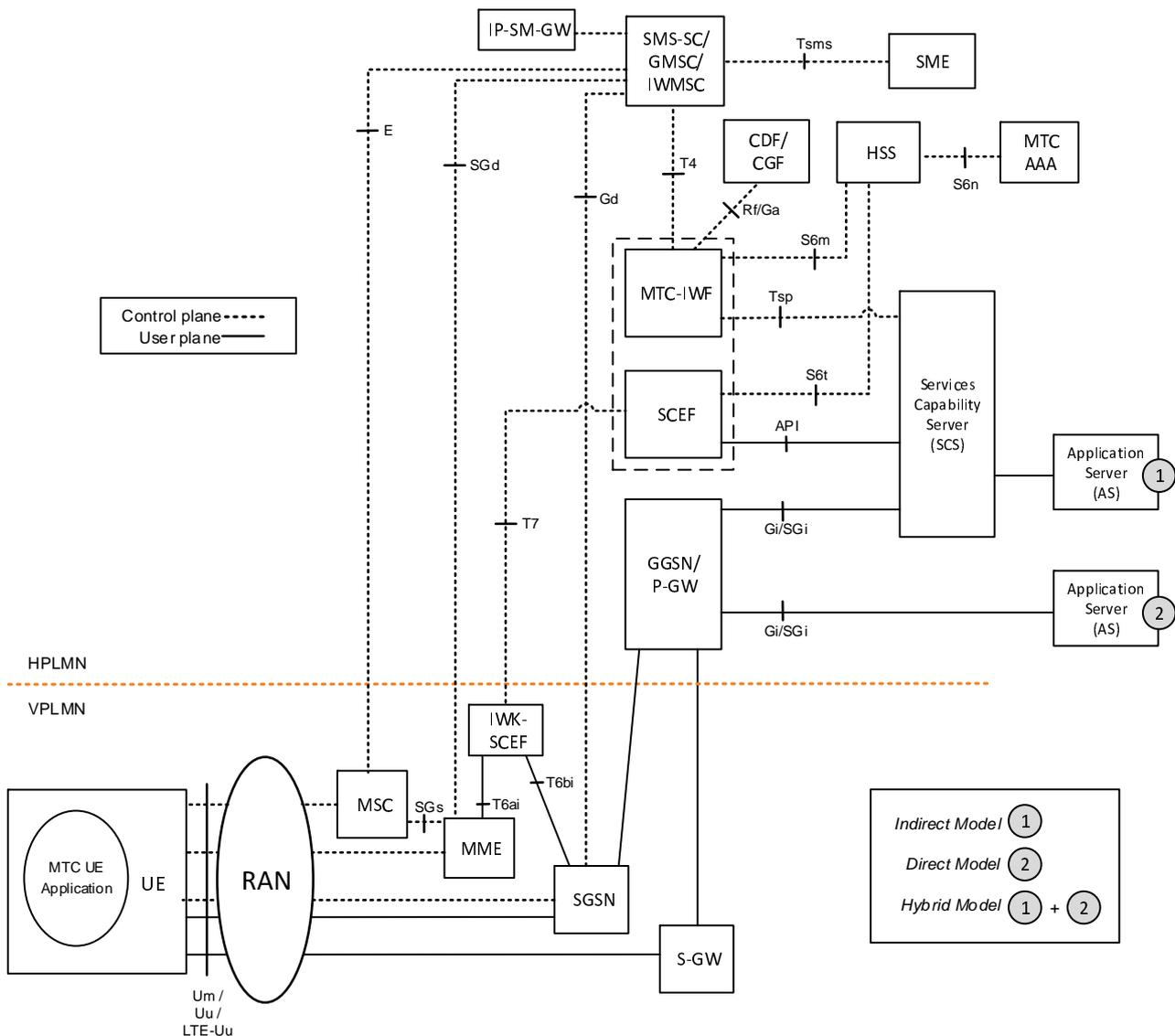
**Figure 4.2-1b: 3GPP Architecture for Machine-Type Communication (Roaming)**
