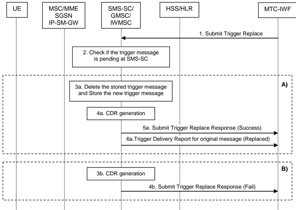
**Figure 5.2.3.2-1: Replace procedure for trigger delivery using T4**
