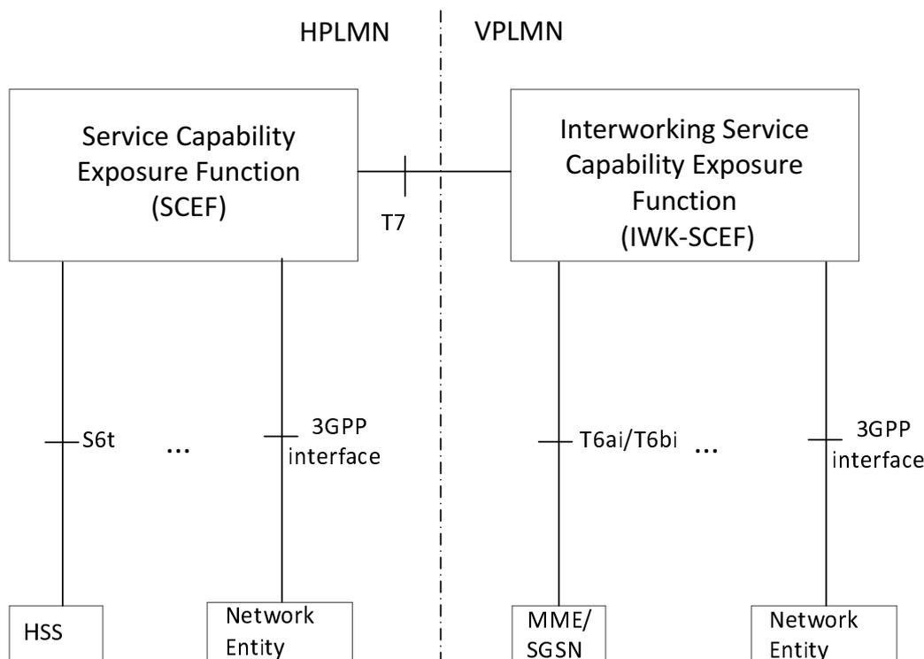
**Figure 4.2-3: 3GPP roaming Architecture for Service Capability Exposure**
