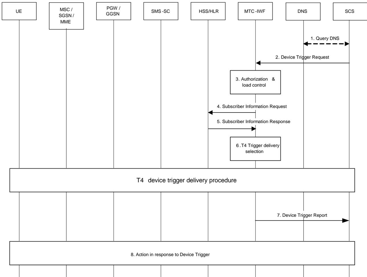
**Figure 5.2.1-1: Device triggering procedure over Tsp**
