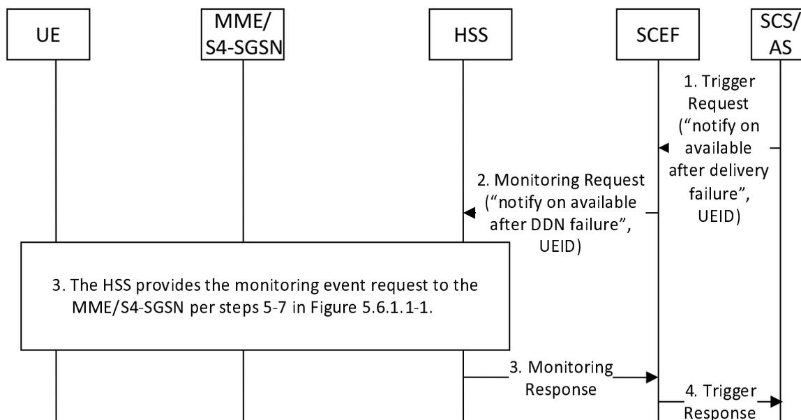
**Figure 5.7.1.2-1: Event Configuration - Availability Notification after DDN Failure**
