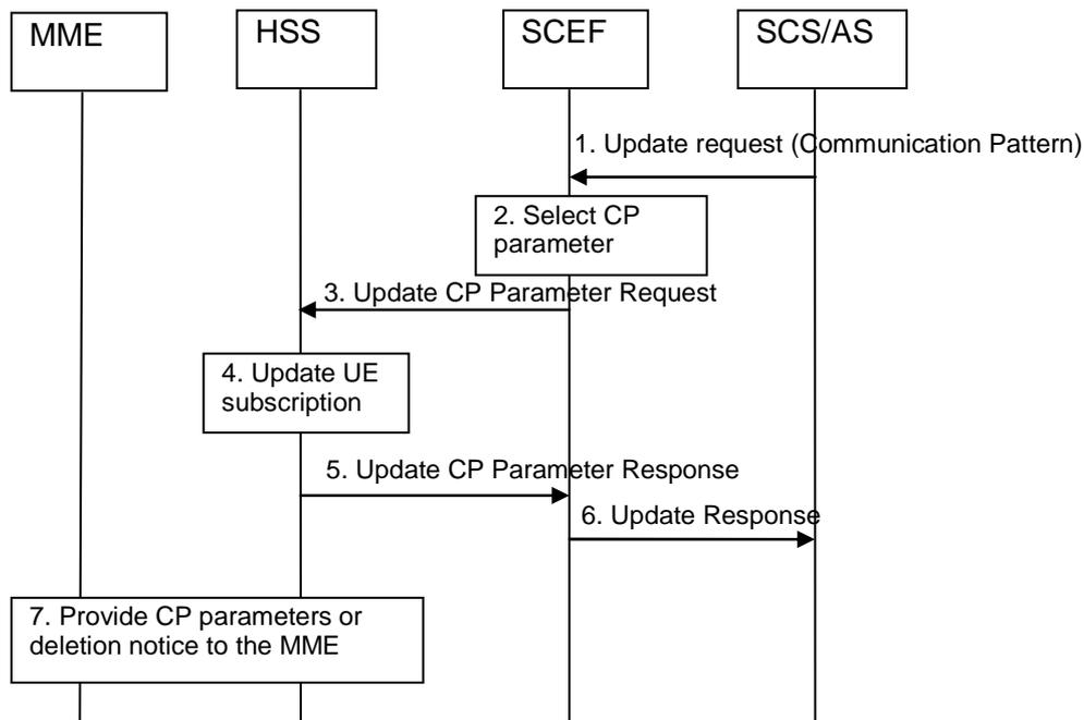
**Figure 5.10.2-1: Signalling sequence for provisioning of CP Parameters**
