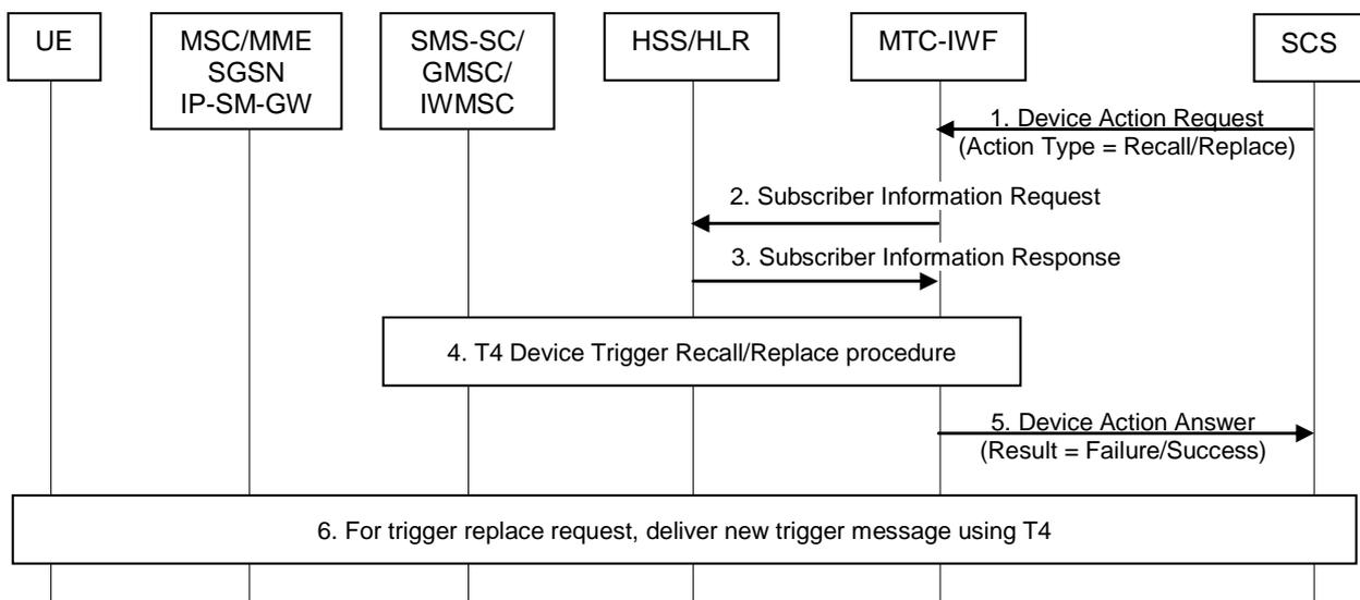
Figure 5.2.3.1-1: Device trigger recall/replace procedure over Tsp
