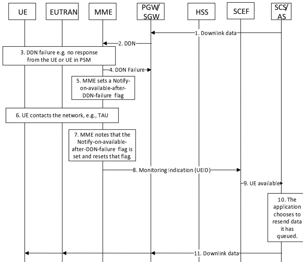
**Figure 5.7.1.3-1: Notification - Availability Notification after DDN Failure**
