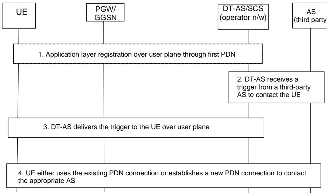
**Figure D-1: Triggering flow using direct model over user plane**
