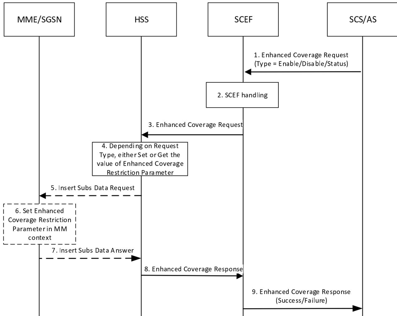
**Figure 5.1-1: Procedure for Enhanced Coverage Restriction Control via SCEF**
