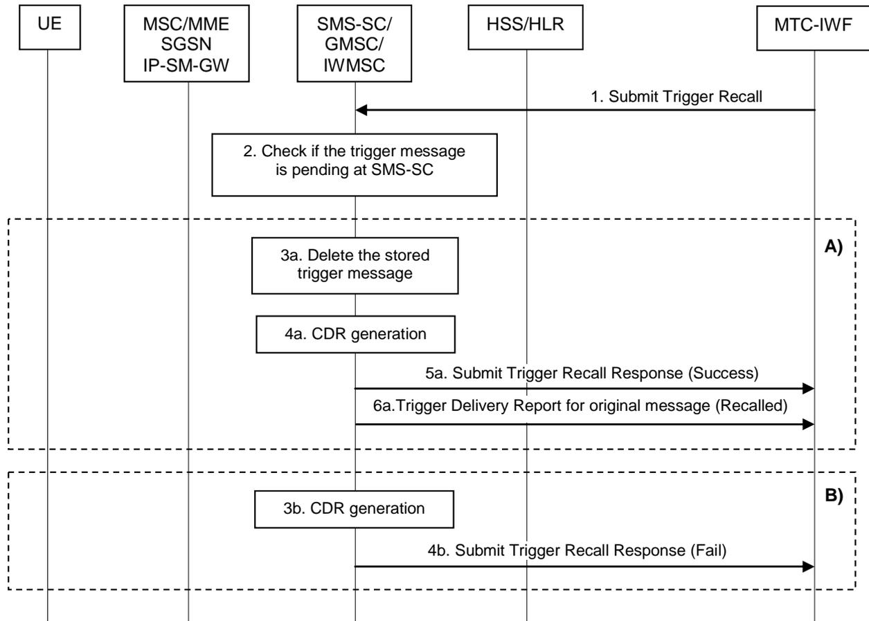
Figure 5.2.3.3-1: Recall procedure for trigger delivery using T4
