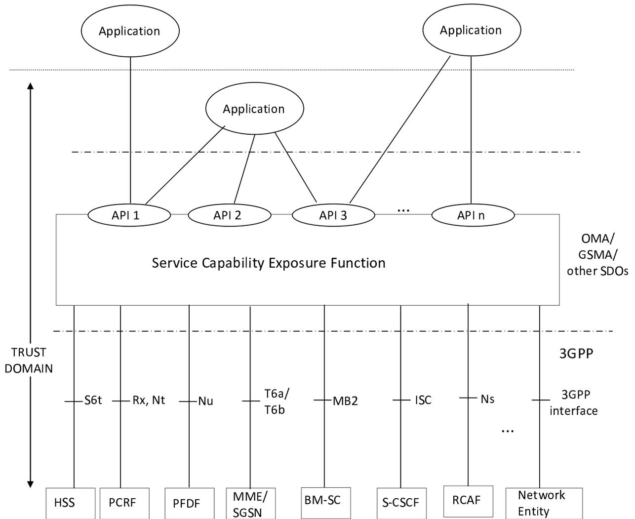
Figure 4.2-2: 3GPP Architecture for Service Capability Exposure
