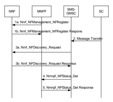
Figure 5.1.7.2-1: GPSI-to-Subscription-Network resolution triggered by the SMS-GMSC
