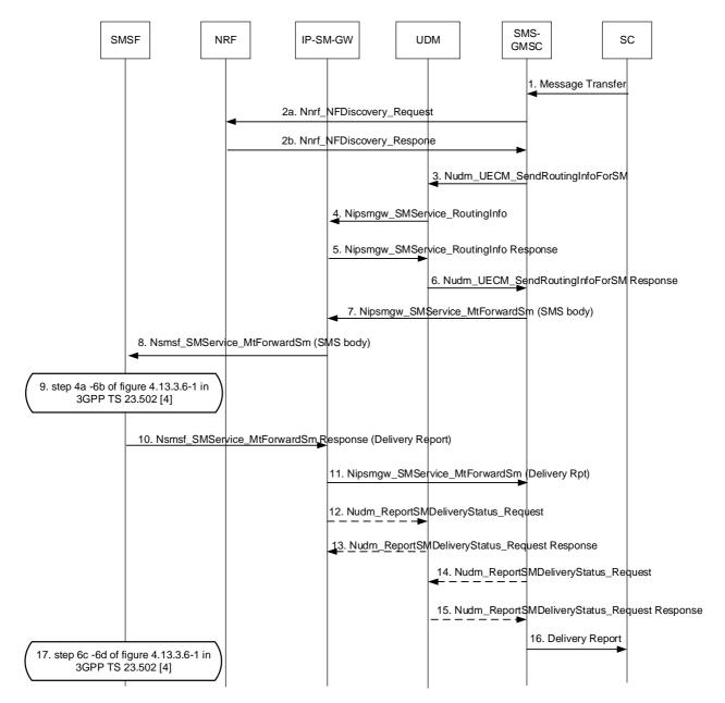
Figure 5.1.4-1: MT SMS over NAS via IP-SM-GW
