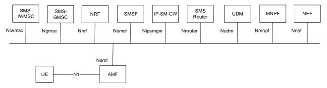
Figure 4.1-1: Non-roaming System Architecture for SBI-based SMS
