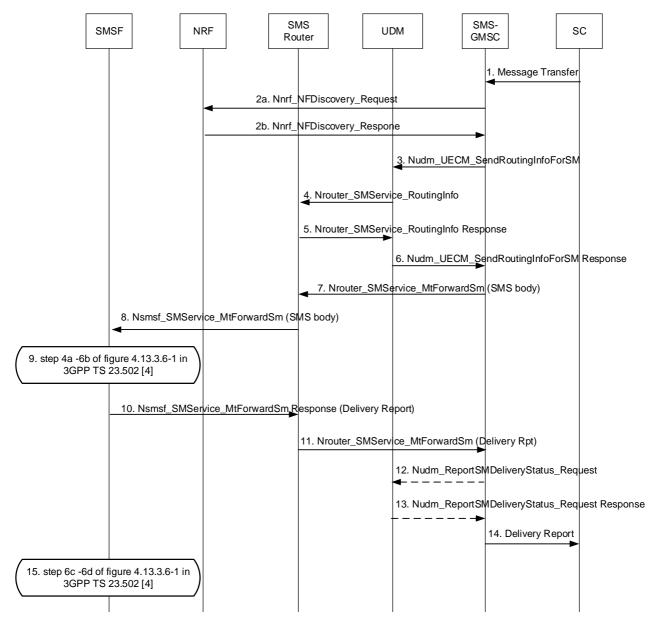
Figure 5.1.3-1: MT SMS over NAS via SMS Router
