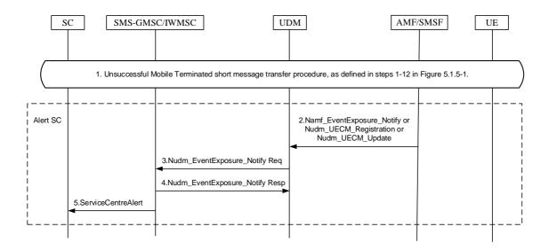
Figure 5.1.8-1: Procedure for alert
