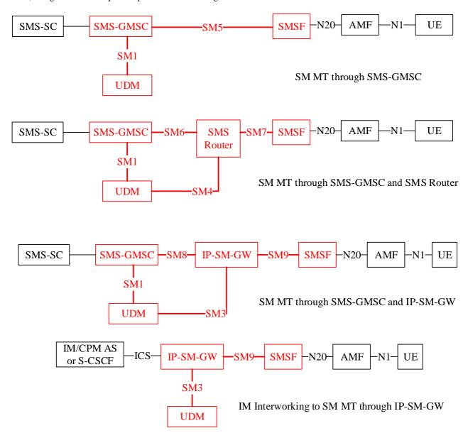
Figure 4.1-2a: Non-roaming System Architecture for SBI-based MT SMS in reference point representation
