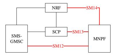
Figure 4.1-2d: Architecture for NP staute Retrival from MNPF in reference point representation
