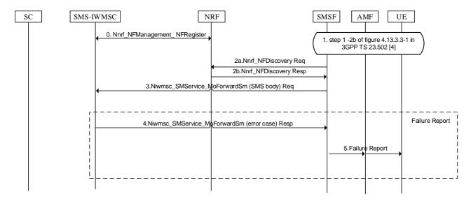
Figure 5.2.3-1: Procedures for unsuccessful SBI-based SM MO message transfer
