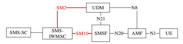
Figure 4.1-2b: Non-roaming System Architecture for SBI-based MO SMS in reference point representation
