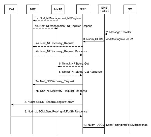
Figure 5.1.7.3.2-1: SCP supports GPSI-to-Subscription-Network resolution with MNPF
