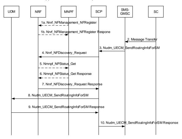
Figure 5.1.7.3.3-1: SCP supports GPSI-to-Subscription-Network resolution with NRF
