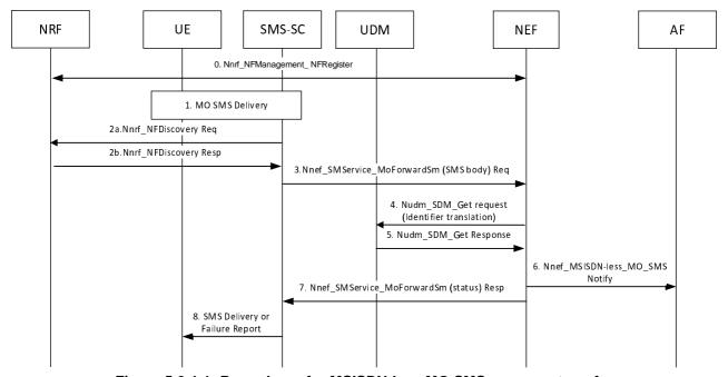
Figure 5.2.4-1: Procedures for MSISDN-less MO SMS message transfer
