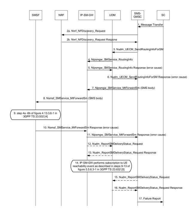
Figure 5.1.6-1: Unsuccessful MT SMS over NAS via IP-SM-GW
