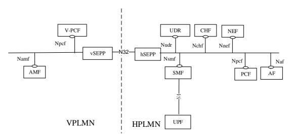
Figure 5.2.2-2: Overall roaming reference architecture of policy and charging control framework for the 5G System - home routed scenario
