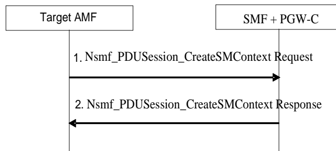
Figure 4.11.1.4.2-1: Procedures for EPS bearer IDs transfer
