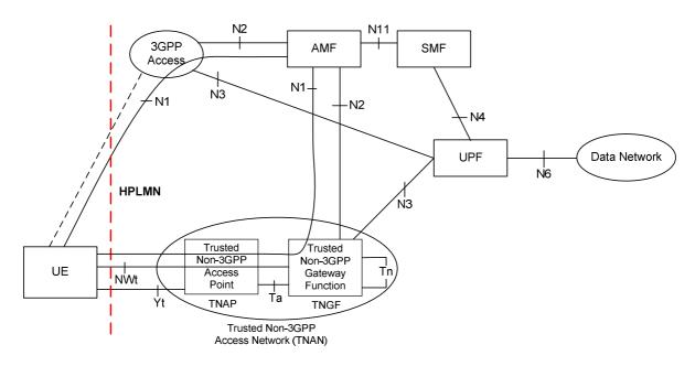
Figure 4.2.8.2.1-2: Non-roaming architecture for 5G Core Network with trusted non-3GPP access
