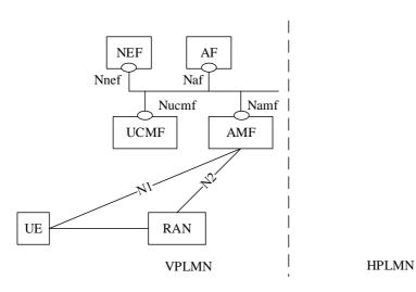
NOTE: The AF in the VPLMN (i.e. the one having a relationship with the VPLMN NEF) is the one which provisions Manufacturer Assigned UE radio capability IDs in the VPLMN UCMF. RACS is a serving PLMN only feature (it requires no specific support in the roaming agreement with the UE HPLMN to operate).
