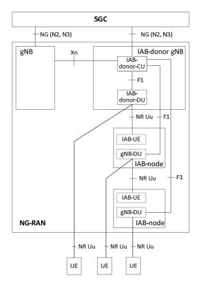
Figure 5.35.1-1: IAB architecture for 5GS
