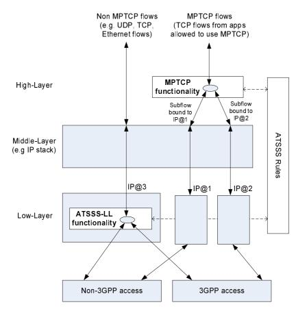
Figure 5.32.6.1-1: Steering functionalities in an example UE model
