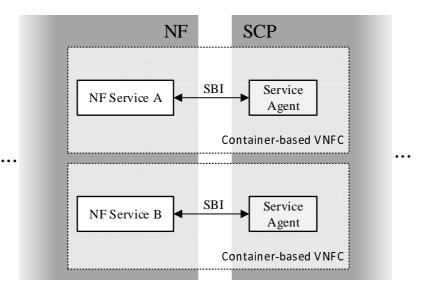
Figure G.2.1-3: Detail of the NF-SCP boundary
