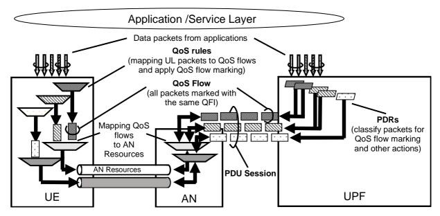
Figure 5.7.1.5-1: The principle for classification and User Plane marking for QoS Flows and mapping to AN Resources
