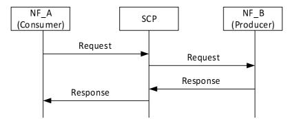
Figure 7.1.2-4: Request response using Indirect Communication
