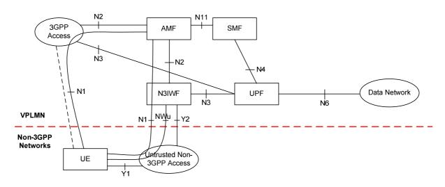
Figure 4.2.8.2.2-1: LBO Roaming architecture for 5G Core Network with untrusted non-3GPP access - N3IWF in the same VPLMN as 3GPP access
