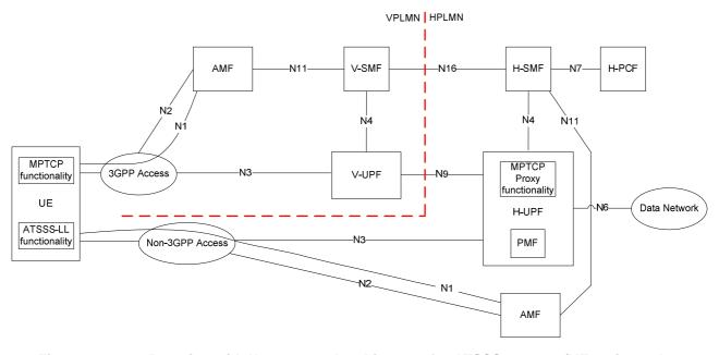
Figure 4.2.10-3: Roaming with Home-routed architecture for ATSSS support (UE registered to different PLMNs)
