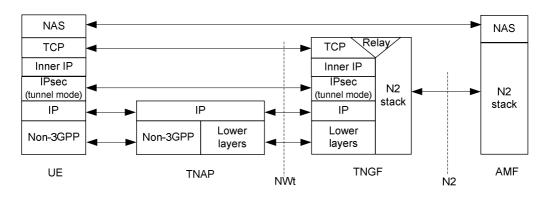
Figure 8.2.5-2: Control Plane after the NWt connection is established between UE and TNGF
