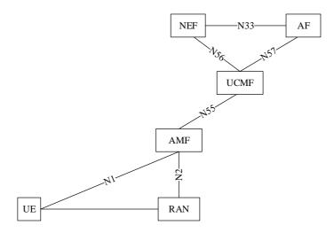
Figure 4.2.5a-1: Radio Capability Signalling optimisation architecture
