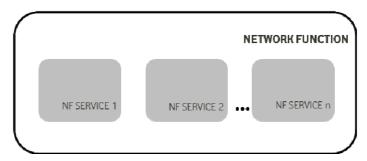
Figure 7.2.1-1: Network Function and NF Service
