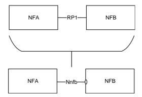
Figure A-2: Example showing a Reference Point replaced by a single Service based Interface
