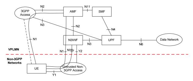
Figure 4.2.8.2.2-1: LBO Roaming architecture for 5G Core Network with non-3GPP access - N3IWF in the VPLMN
