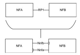
Figure A-1: Example show a Reference Point replaced by two Service based Interfaces
