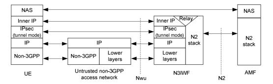
Figure 8.2.4-2: Control Plane after the signalling IPsec SA is established between UE and N3IWF
