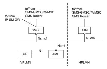
Figure 4.4.2.1-3: Roaming architecture for SMS over NAS
