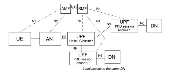
Figure 5.6.4.2-1 User plane Architecture for the Uplink Classifier
