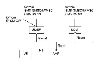
Figure 4.4.2.1-1: Non-roaming System Architecture for SMS over NAS
