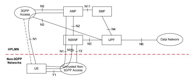
Figure 4.2.8.2.1-1: Non-roaming architecture for 5G Core Network with non-3GPP access
