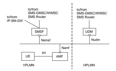
Figure 4.4.2.1-3: Roaming architecture for SMS over NAS
