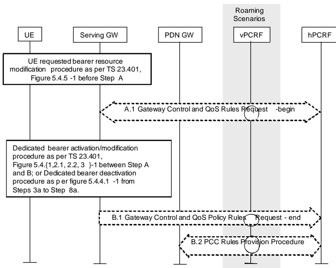
**Figure 5.5-1: UE-initiated resource request/release with PMIP-based S5/S8**
