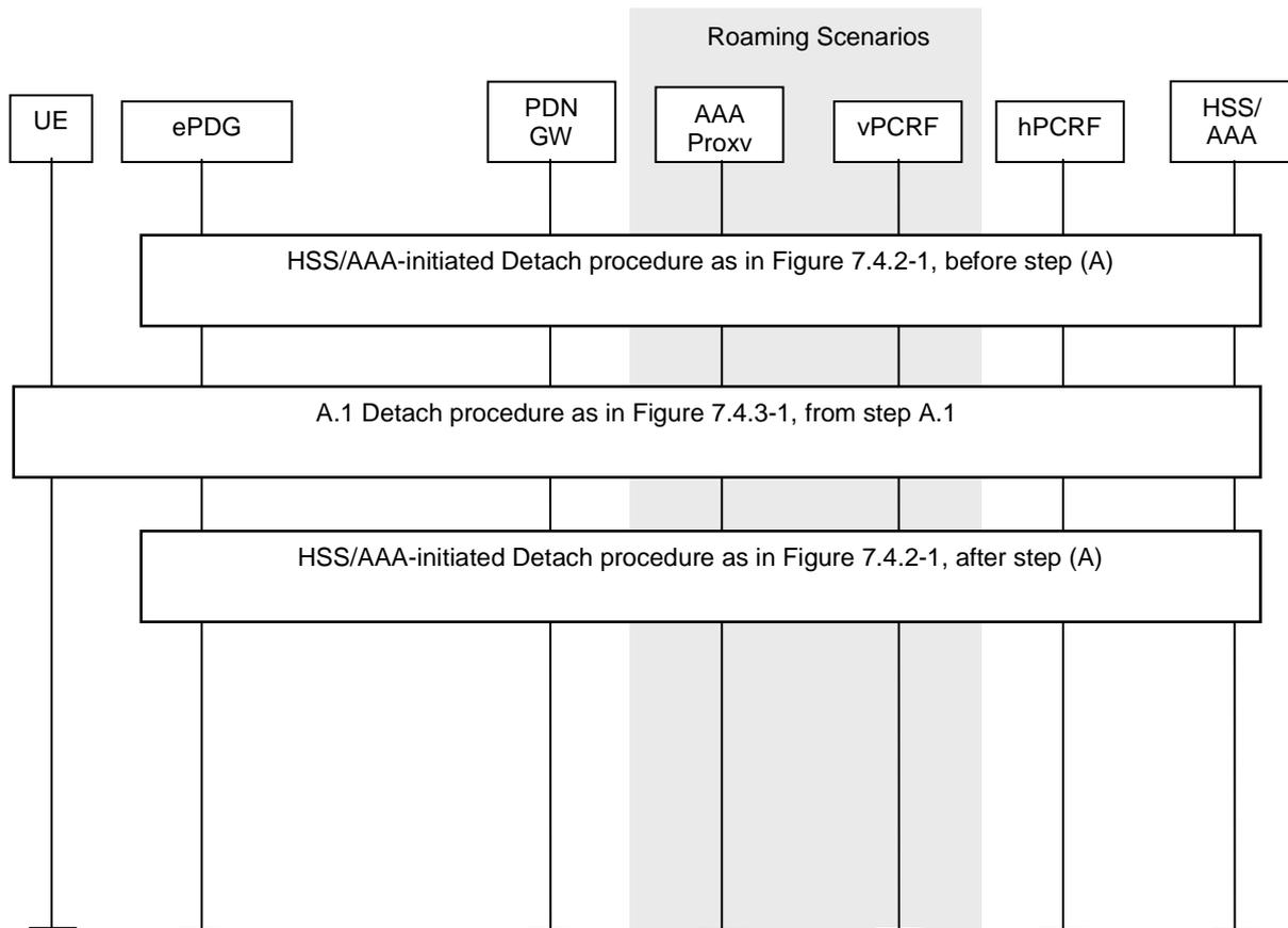
**Figure 7.4.4-1: HSS/AAA-initiated detach procedure with GTP on S2b**
