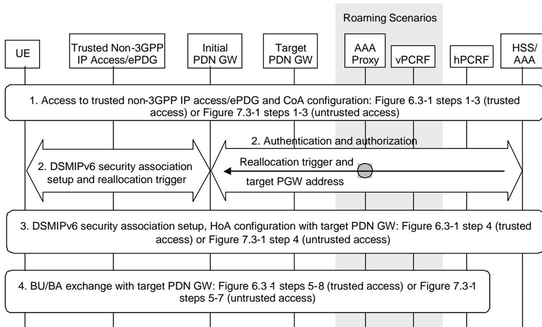
**Figure 6.10-1: PDN GW reallocation upon attach on S2c**
