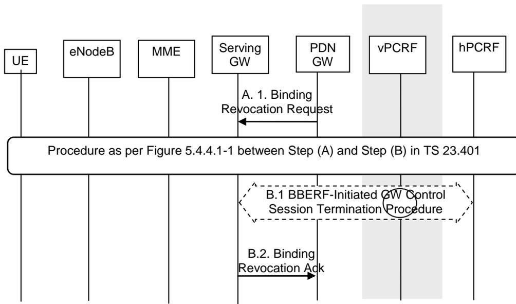
**Figure 5.6.2.2-1: PDN GW initiated PDN Disconnection Procedure for PMIP-based S5/S8**
