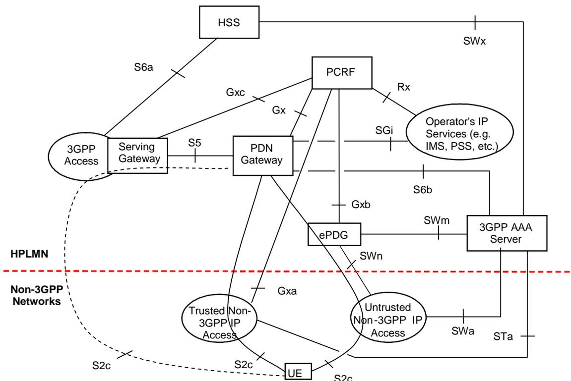
Figure 4.2.2-2: Non-Roaming Architecture within EPS using S5, S2c
