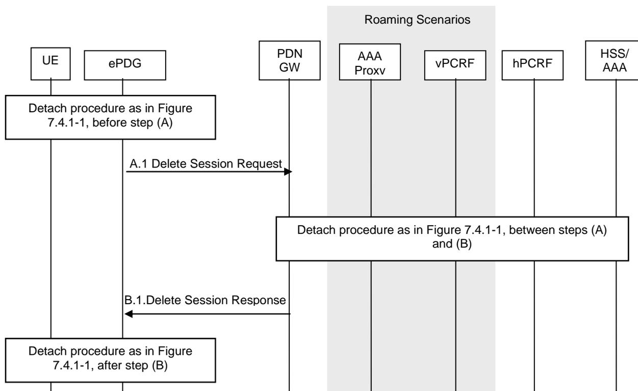
**Figure 7.4.3-1: UE/ePDG-initiated detach procedure with GTP on S2b**
