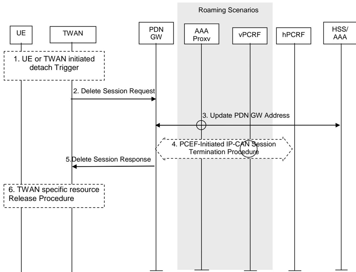
**Figure 16.7.1.1-1: UE/TWAN-Initiated Detach in WLAN on GTP S2a**
