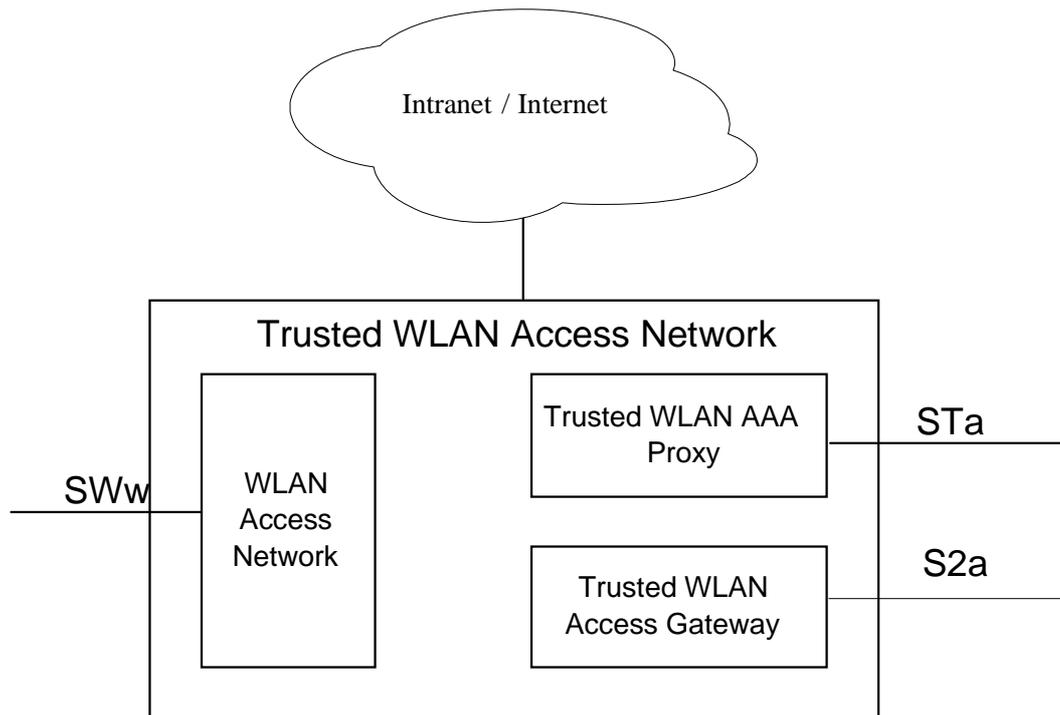
**Figure 16.1.2-1: Trusted WLAN Access Network functional split**
