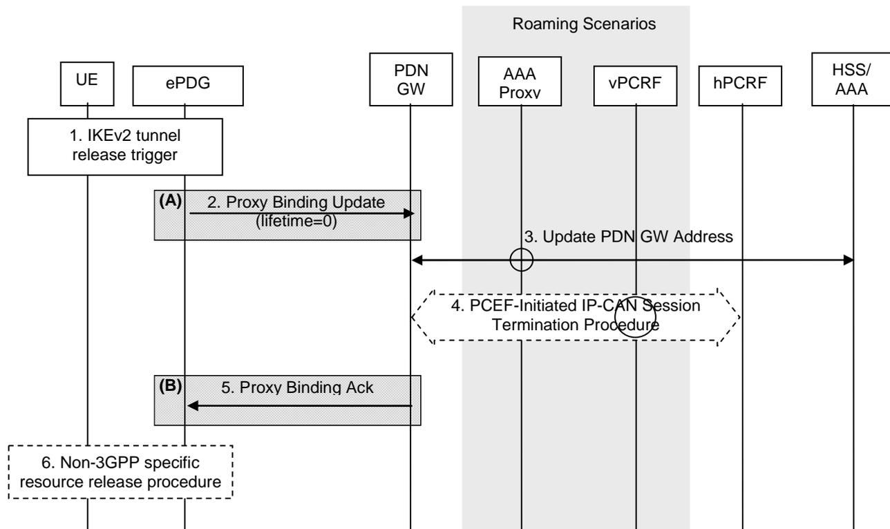
**Figure 7.4.1-1: UE/ePDG-initiated detach procedure with PMIPv6 on S2b**
