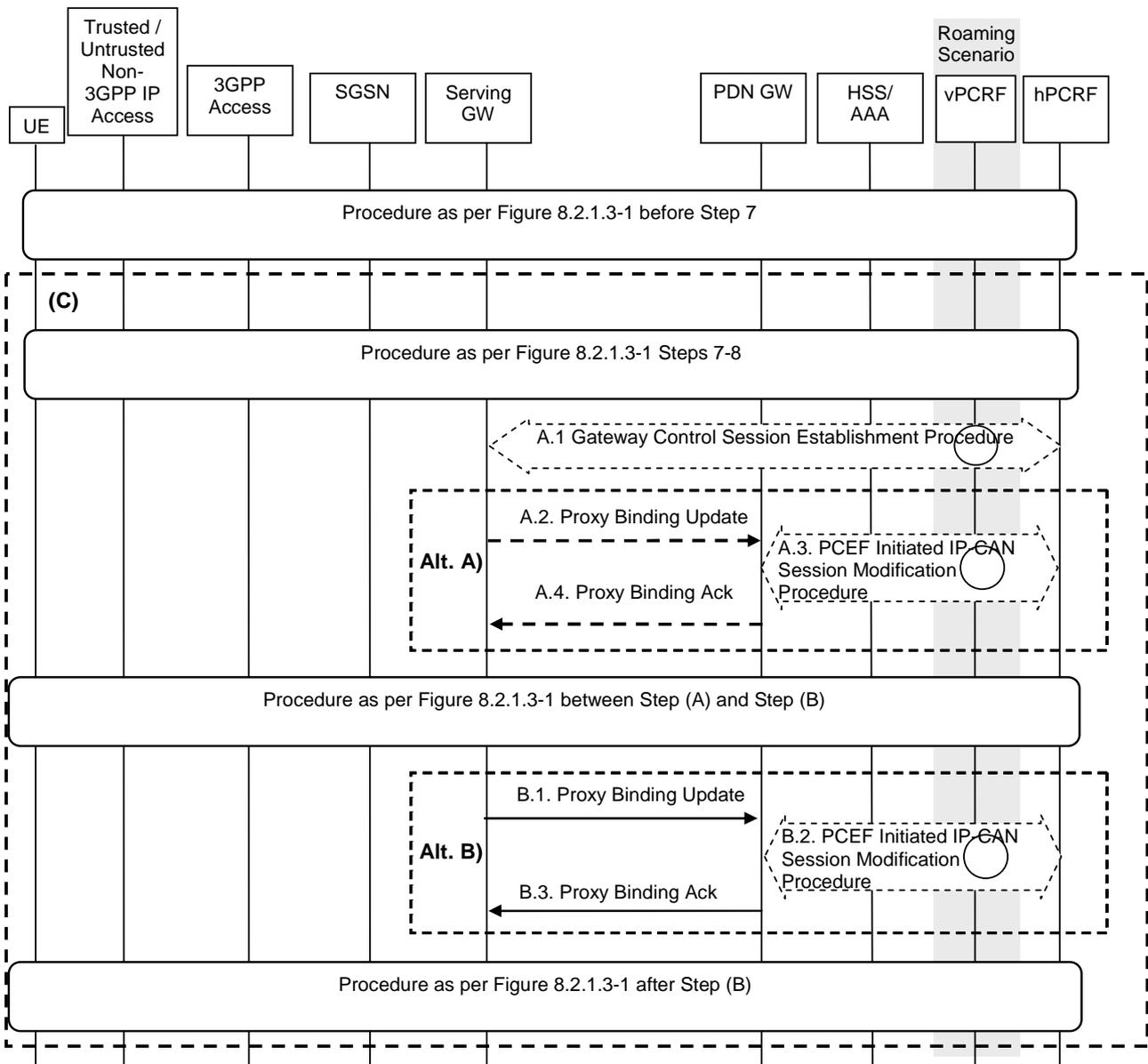
Figure 8.2.1.4-1: Trusted/untrusted Non-3GPP IP Access to GERAN/UTRAN over PMIP-based S2a and using PMIP-based S5/S8
