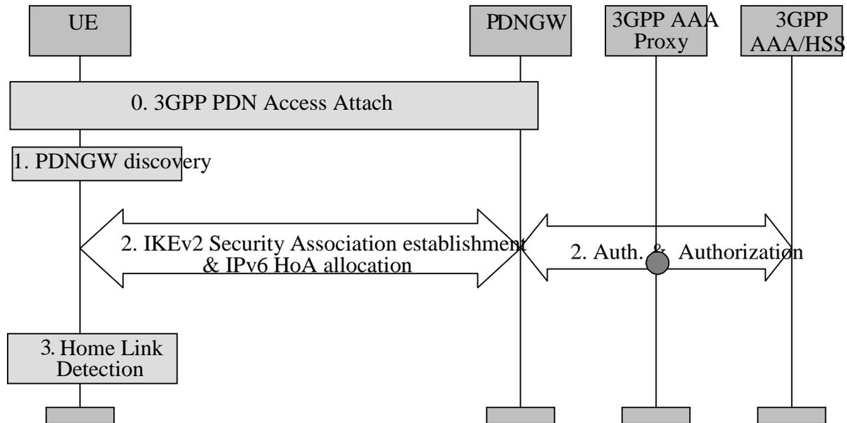
**Figure 15.1-1: S2c PDN Attach via DSMIPv6 home link**
