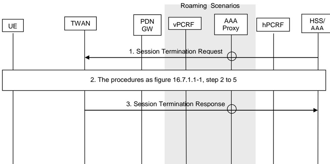
Figure 16.7.1.2-1: HSS/AAA-Initiated Detach in WLAN on GTP S2a
