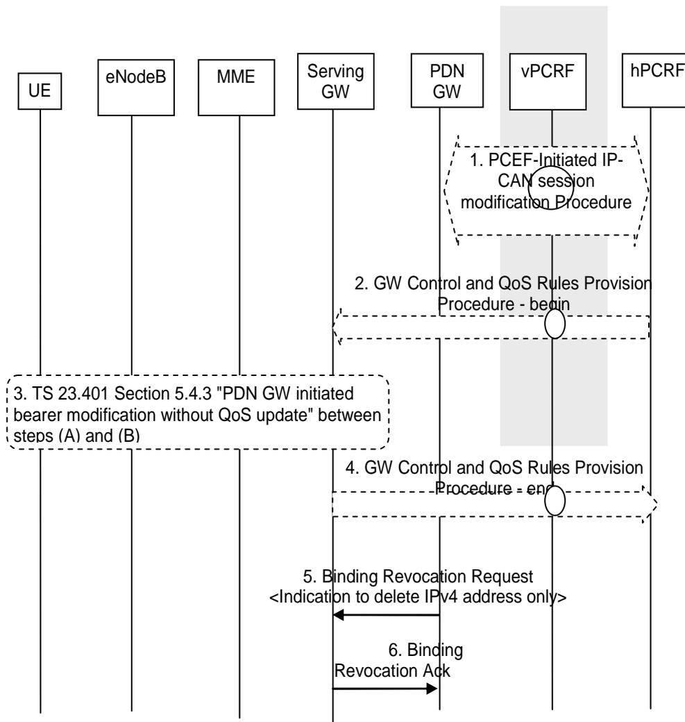
**Figure 5.11-1: PDN GW initiated IPv4 address Delete Procedure**
