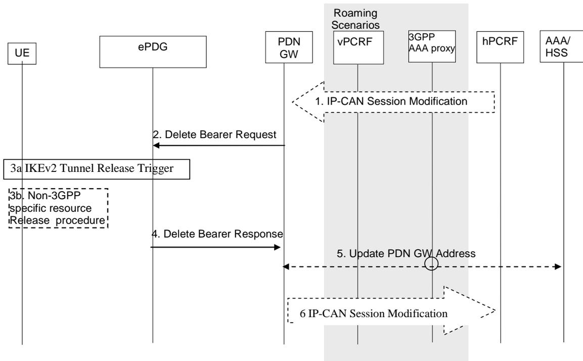
**Figure 7.9.2-1: PDN GW Initiated Bearer Deactivation with GTP on S2b**
