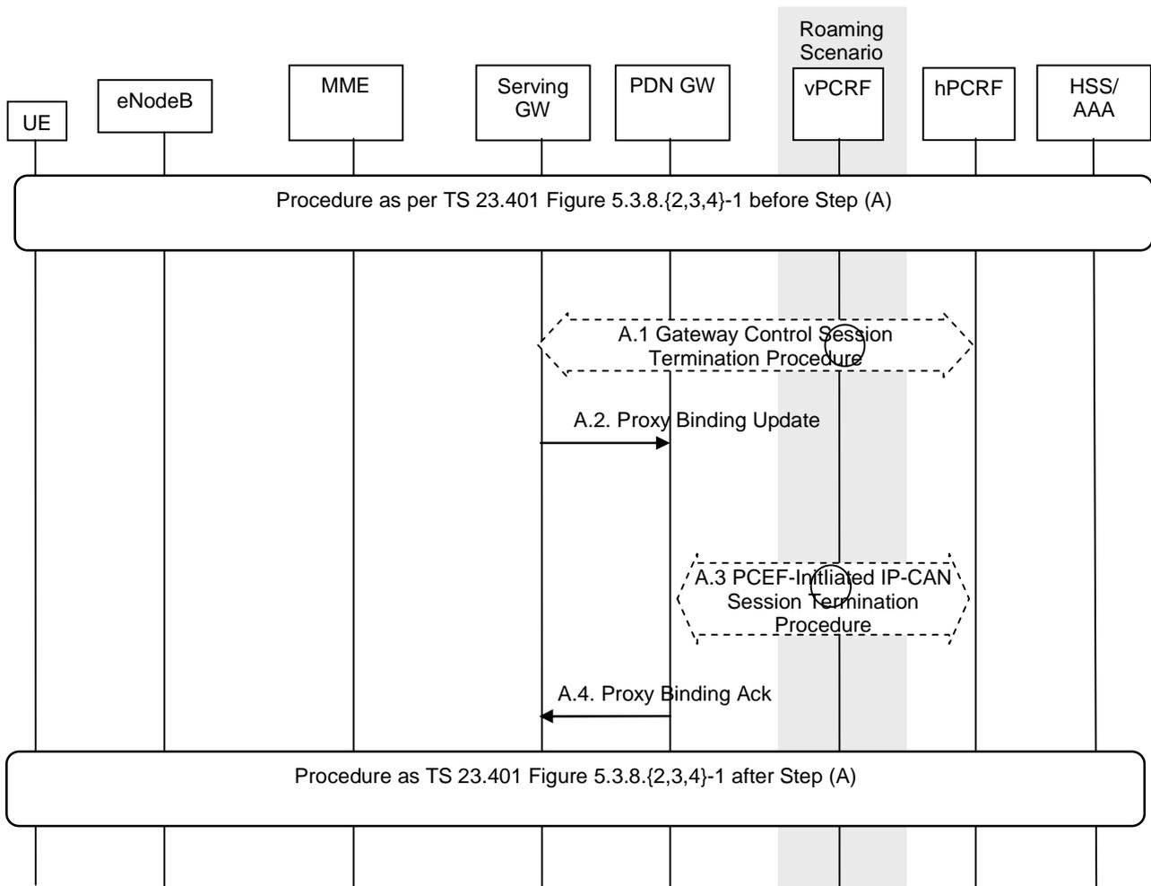
**Figure 5.3-1: E-UTRAN Detach Procedure for PMIP-based S5/S8**
