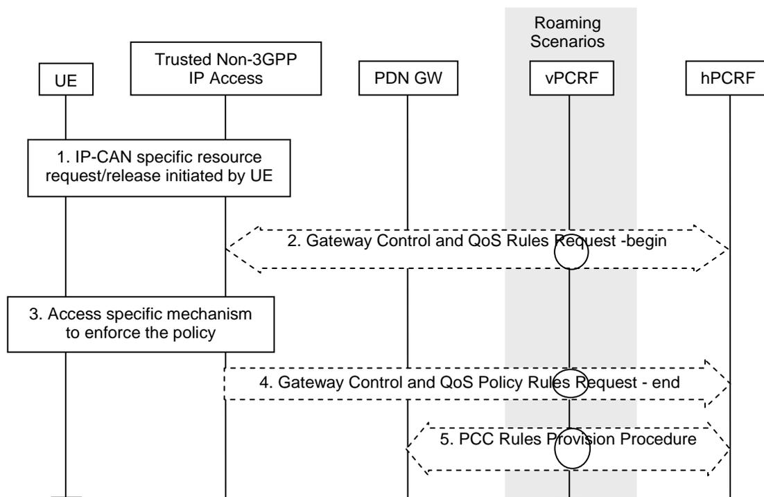
**Figure 6.7.1-1: UE-initiated resource request/release with S2a or S2c**
