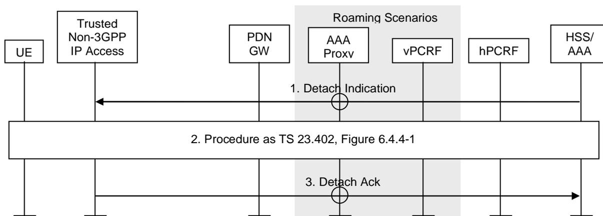
**Figure 6.4.5-1: HSS/AAA-initiated detach procedure with MIPv4 FACoA**
