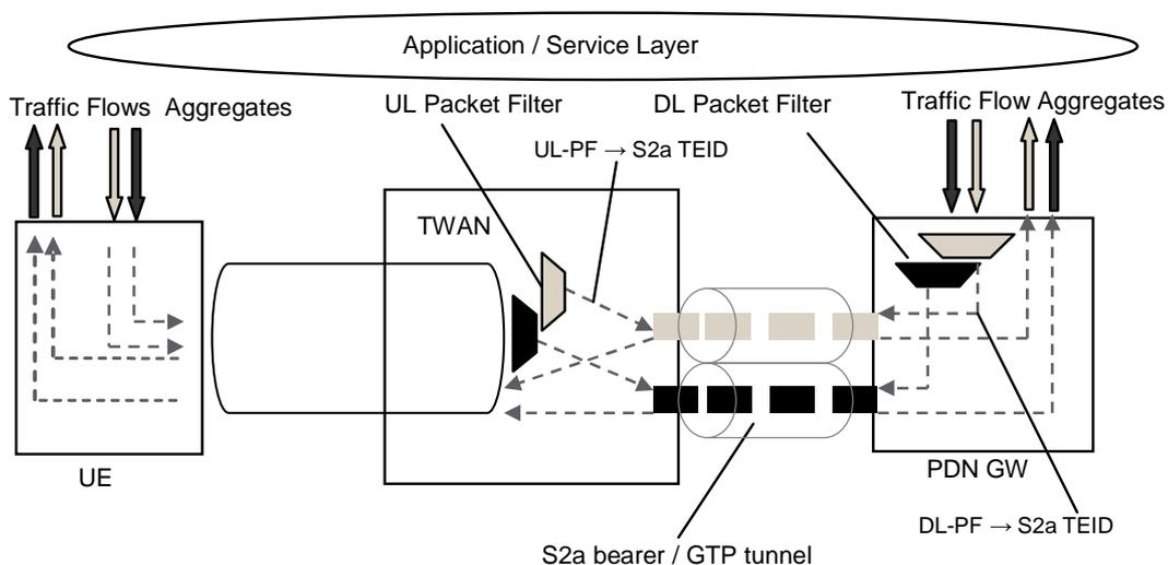
**Figure 16.1.6-1: Two Unicast S2a bearers (GTP based S2a)**
