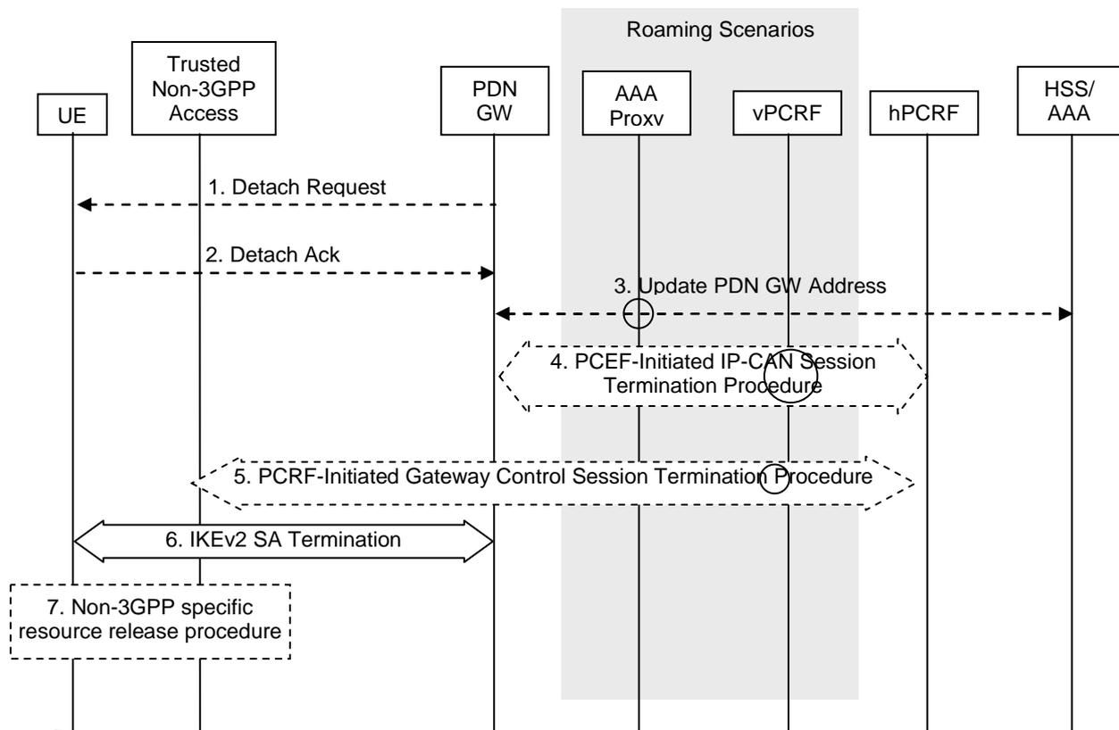
**Figure 6.5.4-1: PDN GW- initiated PDN Disconnection S2c procedure in Trusted Non-3GPP Access Network**
