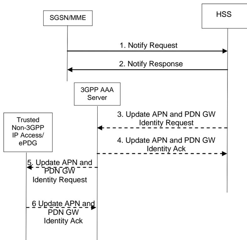
**Figure 12.1.5-1: PDN GW address notification from SGSN/MME**
