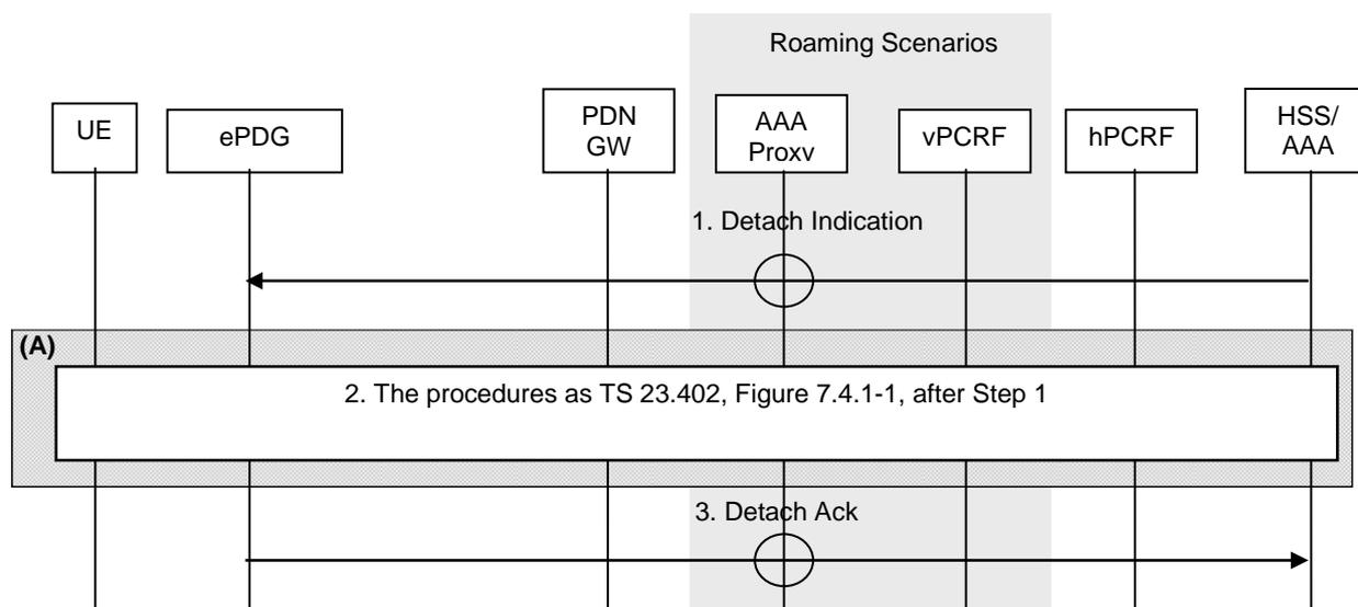
**Figure 7.4.2-1: HSS/AAA-initiated detach procedure with PMIPv6 on S2b**
