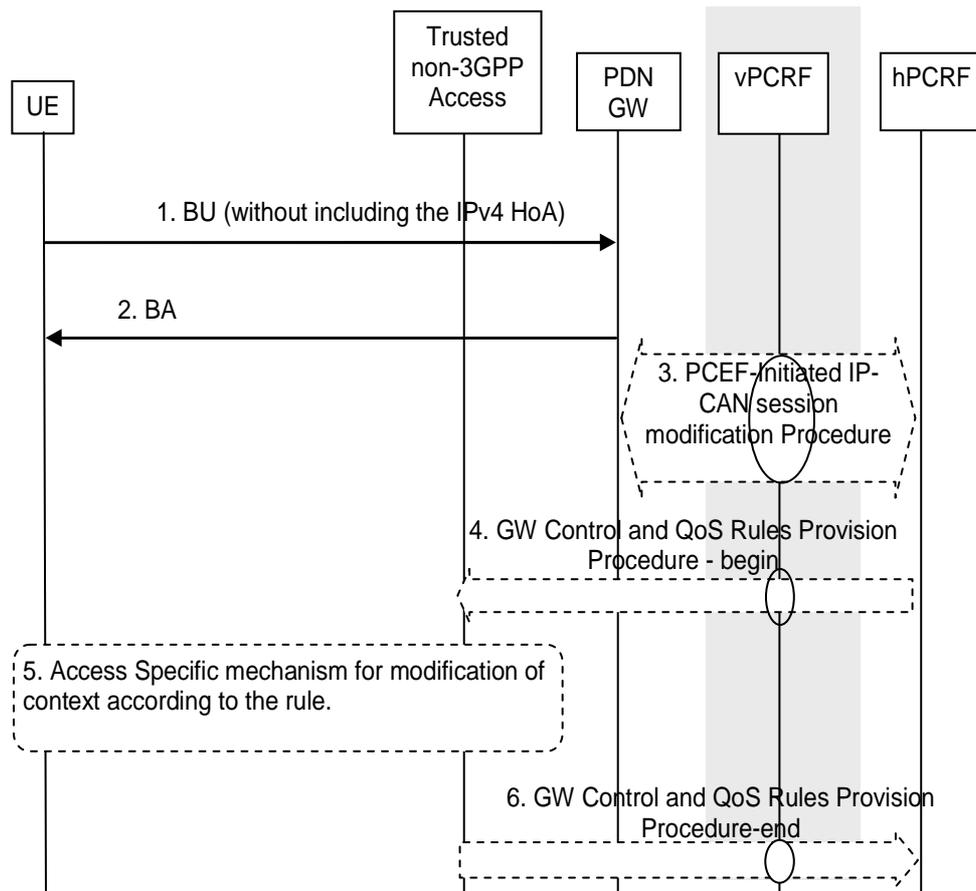
**Figure 6.15-1: IPv4 Home Address Release Procedure for S2c**
