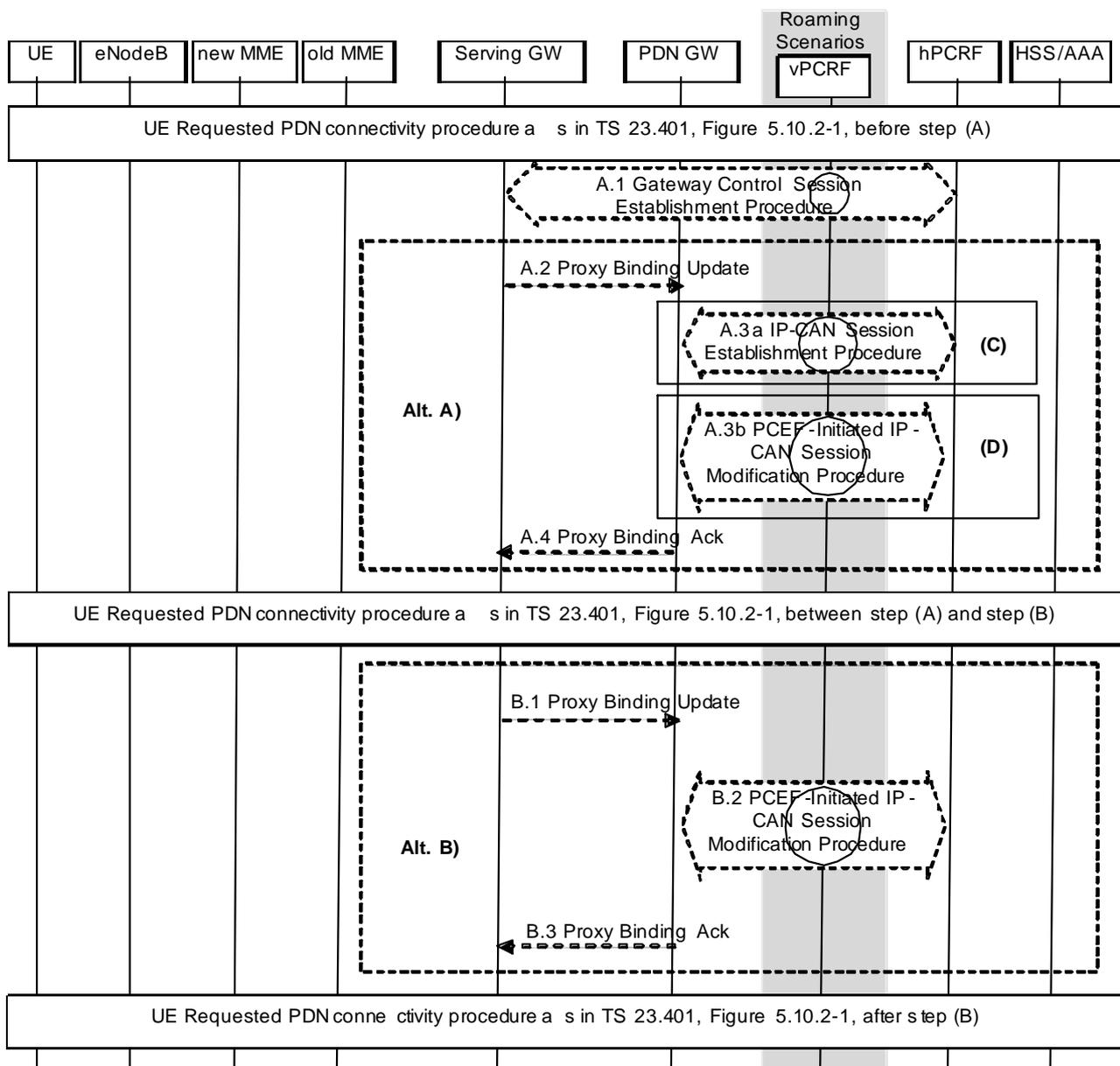
**Figure 5.6.1-1: UE requested PDN connectivity with PMIP-based S5 or S8**
