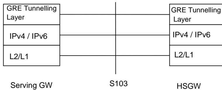
**Figure 9.1.2.6-1: Protocol Stack for the S103 Reference Point**
