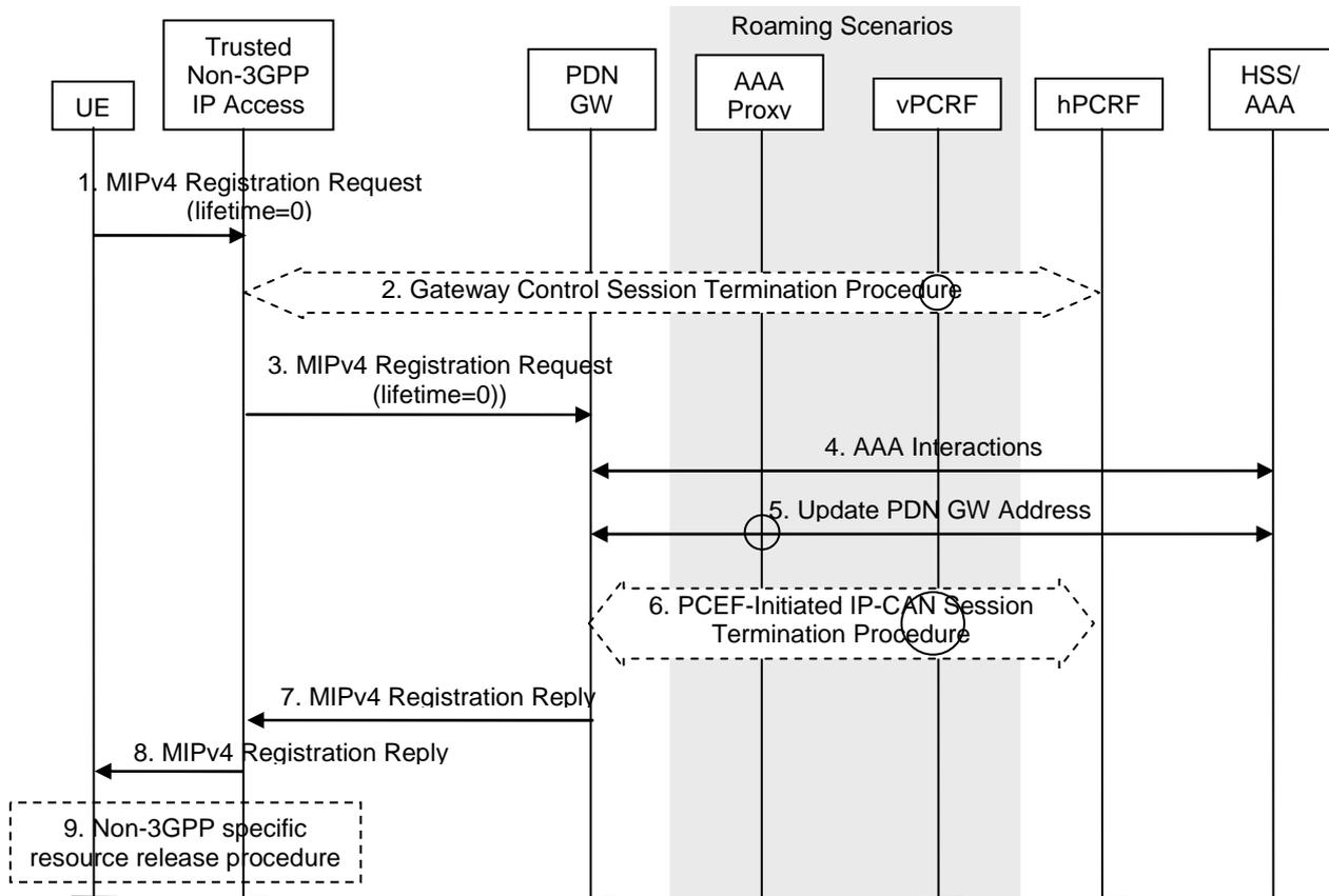
**Figure 6.4.3-1: UE-initiated detach procedure with MIPv4 FACoA**
