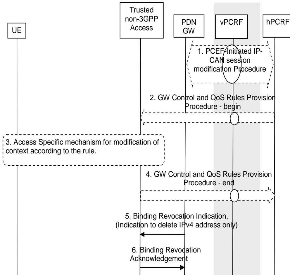
Figure 6.13-1: PDN GW initiated IPv4 address Delete Procedure
