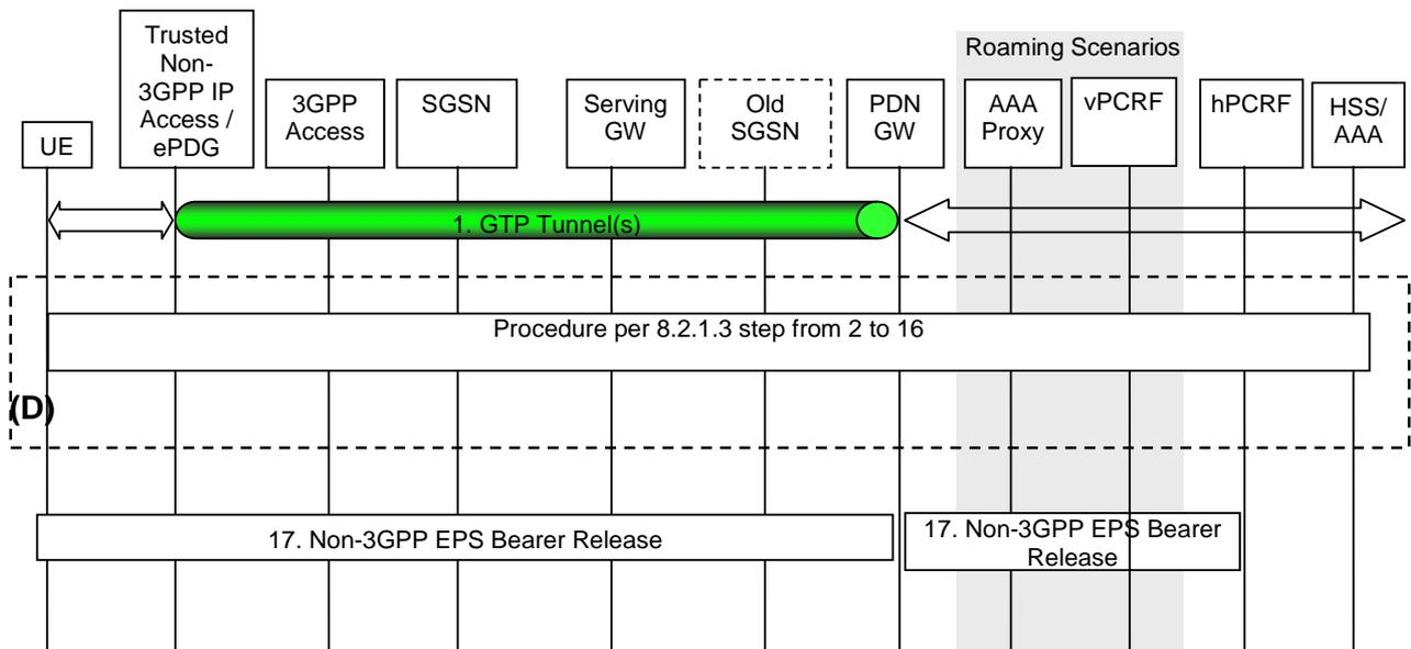
**Figure 8.6.1.2-1: Handover from Untrusted Non-3GPP IP Access to UTRAN/GERAN with GTP on S2b and GTP on S5/S8 interfaces**
