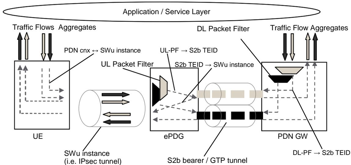
**Figure 4.10.5-1: Two Unicast S2b bearers (GTP based S2b)**
