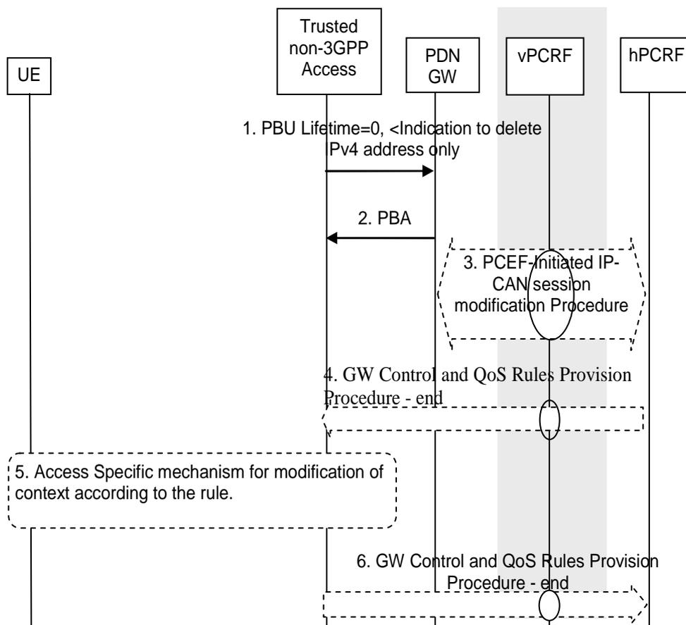
Figure 6.14-1: Non-3GPP access initiated IPv4 address Delete Procedure
