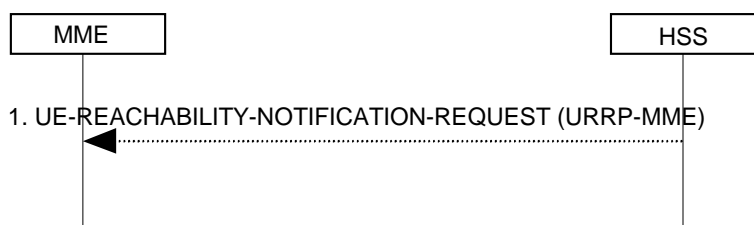
Figure 5.3.11.2-1: UE Reachability Notification Request Procedure
