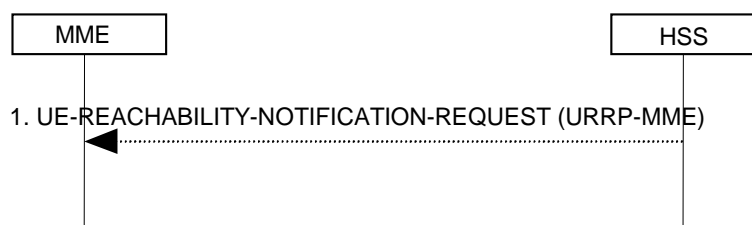
Figure 5.3.11.2-1: UE Reachability Notification Request Procedure
