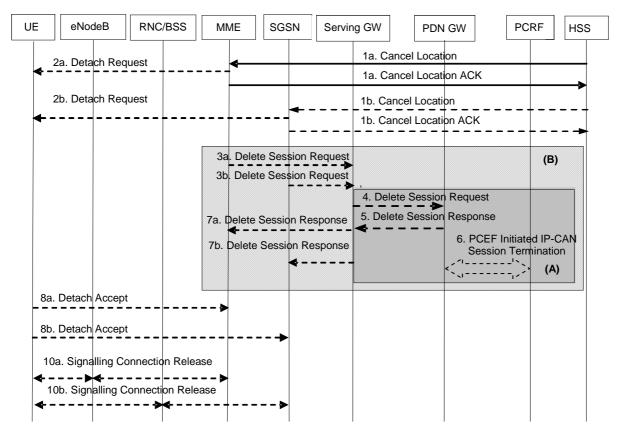
Figure 5.3.8.4-1: HSS-Initiated Detach Procedure
