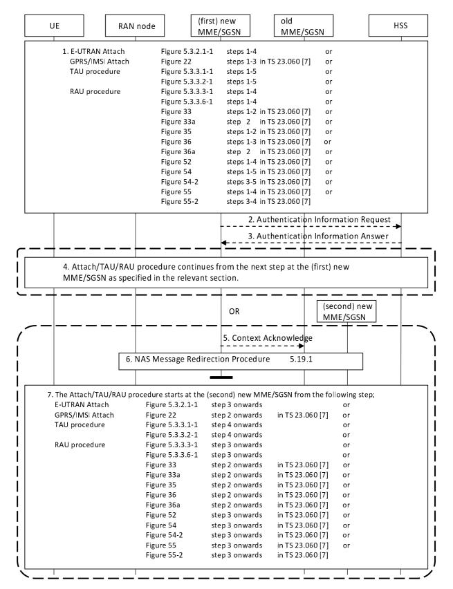
Figure 5.19.2-1: Attach, TAU and RAU procedure for Dedicated Core Network
