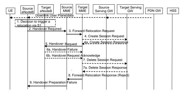
Figure 5.5.1.2.3-1: S1-based handover, Reject
