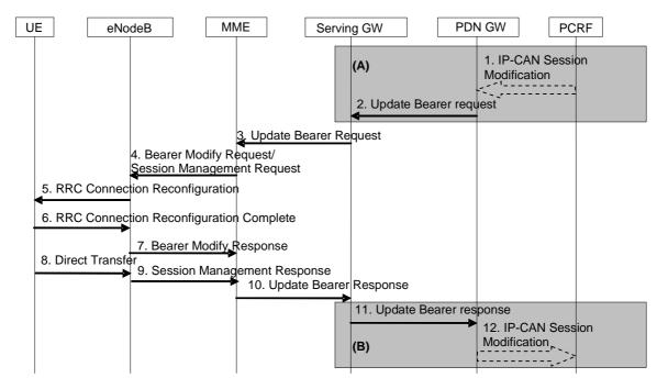
Figure 5.4.2.1-1: Bearer Modification Procedure with Bearer QoS Update
