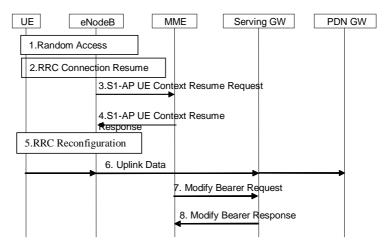
Figure 5.3.5A-1: UE initiated Connection Resume procedure
