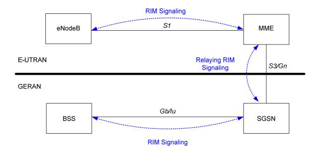
Figure 5.6-1: E-UTRAN to GERAN NACC basic network architecture
