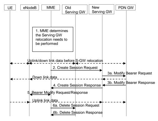
Figure 5.10.4-1: MME triggered Serving GW relocation
