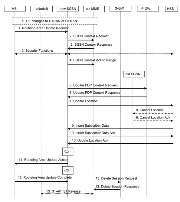
Figure D.3.5-1: Routing Area Update procedure
