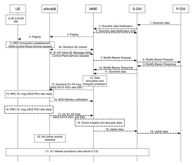
Figure 5.3.4B.3-1: MT Data transport in NAS PDUs
