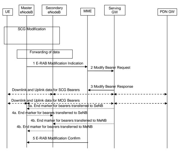
Figure 5.4.7-1: E-UTRAN initiated E-RAB modification procedure
