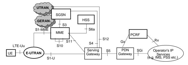
Figure 4.2.1-1: Non-roaming architecture for 3GPP accesses
