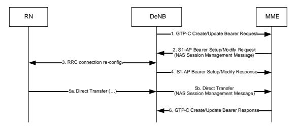
Figure 4.3.20.3-1: DeNB-initiated bearer activation/modification procedure
