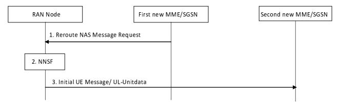
Figure 5.19.1-1: NAS Message Redirection Procedure
