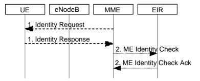
Figure 5.3.10.5-1: Identity Check Procedure
