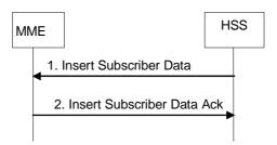
Figure 5.3.9.2-1: Insert Subscriber Data procedure
