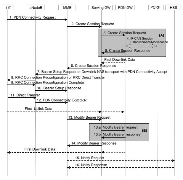
Figure 5.10.2-1: UE requested PDN connectivity
