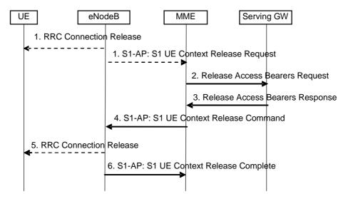
Figure 5.3.5-1: S1 Release Procedure
