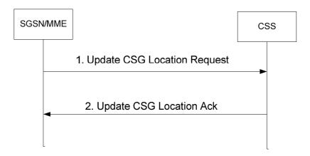
Figure 5.3.12-1: Update CSG Location Procedure
