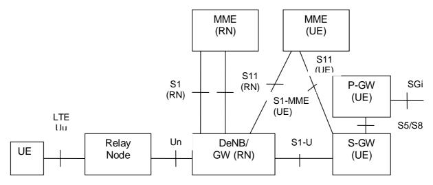
Figure 4.3.20.1-1: Relaying Architecture
